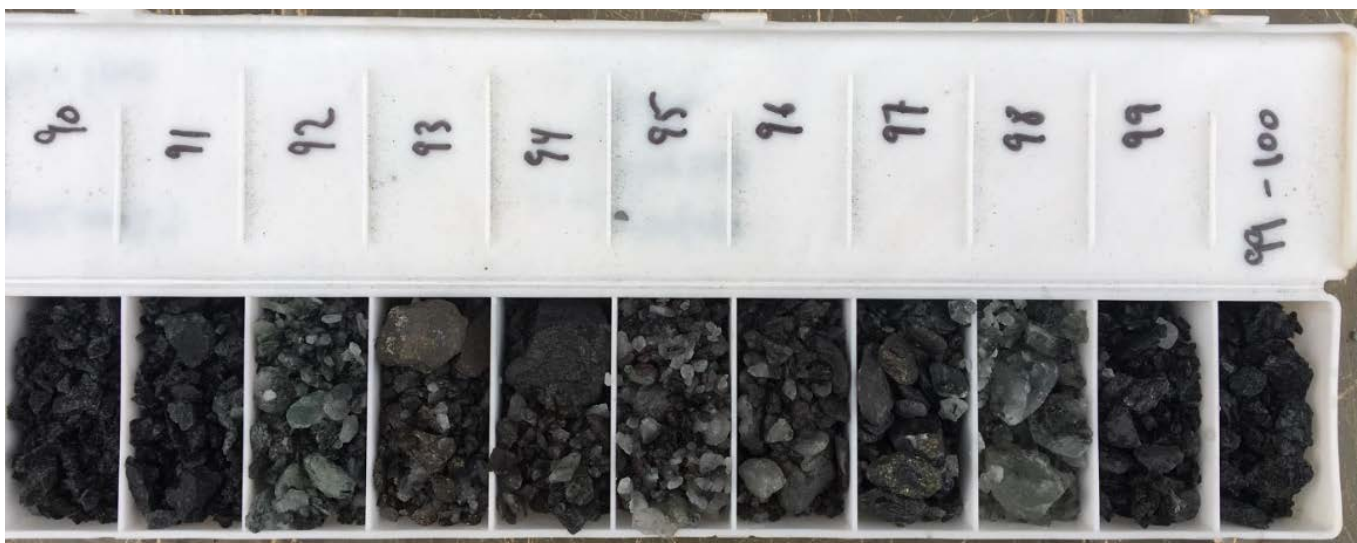
Figure 3: RC drill chips from mineralised zone in DRRC0024 of 7m @ 27.4g/t gold from 92m including 5m @ 37.5 g/t gold from 92m.
