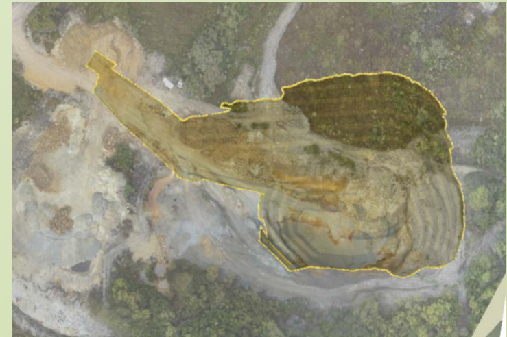
Topographical overview of existing Granville East Mine with proposed east wall cutback superimposed
