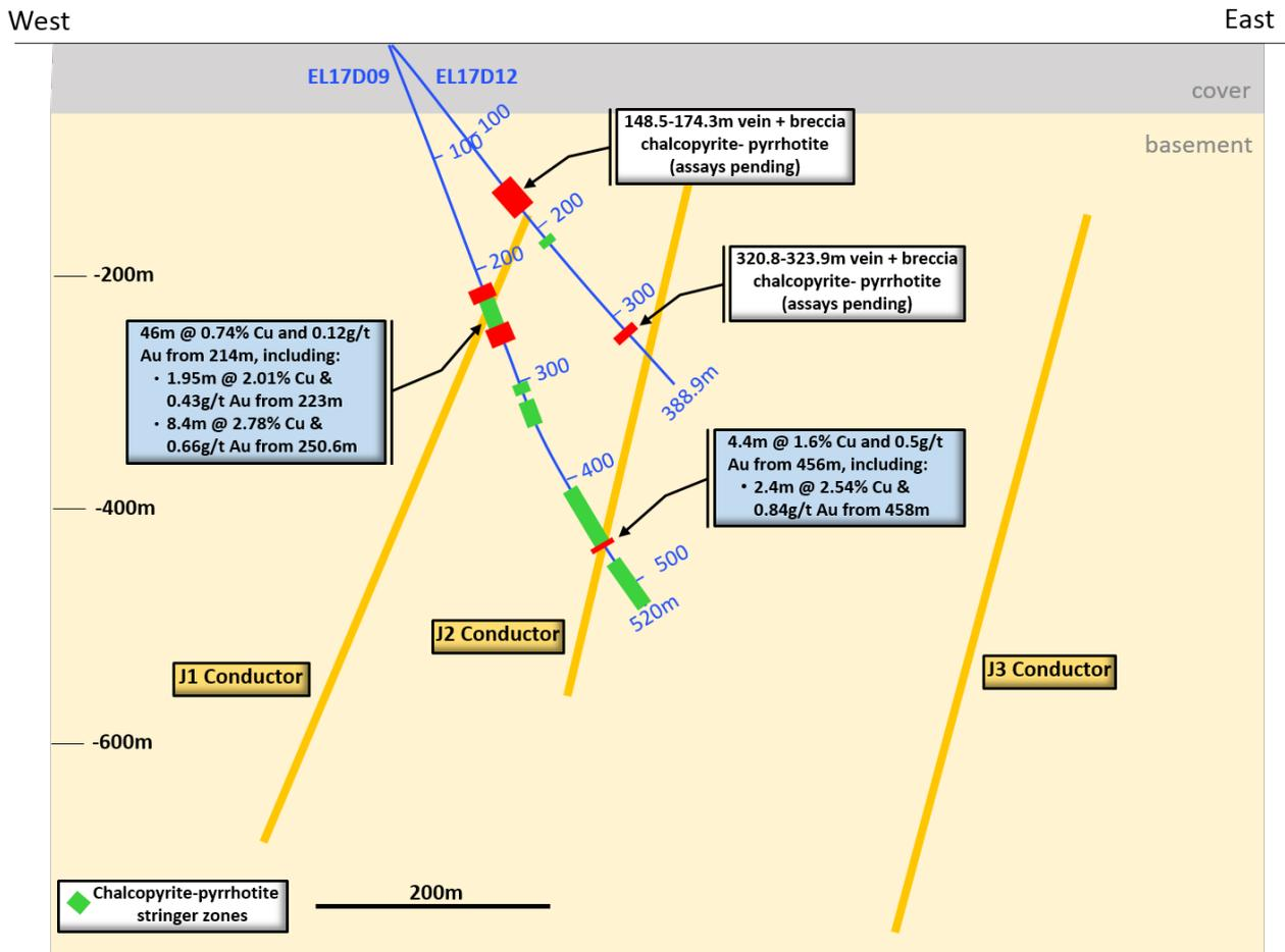
Figure 4: Cross-section (viewed north) at Jericho prospect showing completed drill holes EL17D09 and EL17D12, the 2 modelled EM pleates and zones of copper mineralisation
