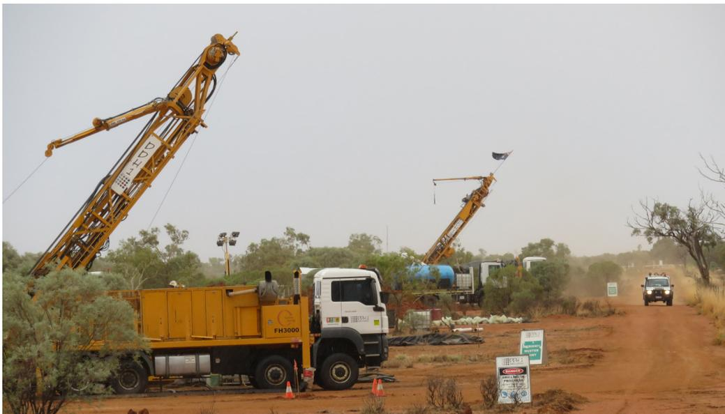
Picture 1: DDH1 diamond rigs drilling 24/7 at Jericho
