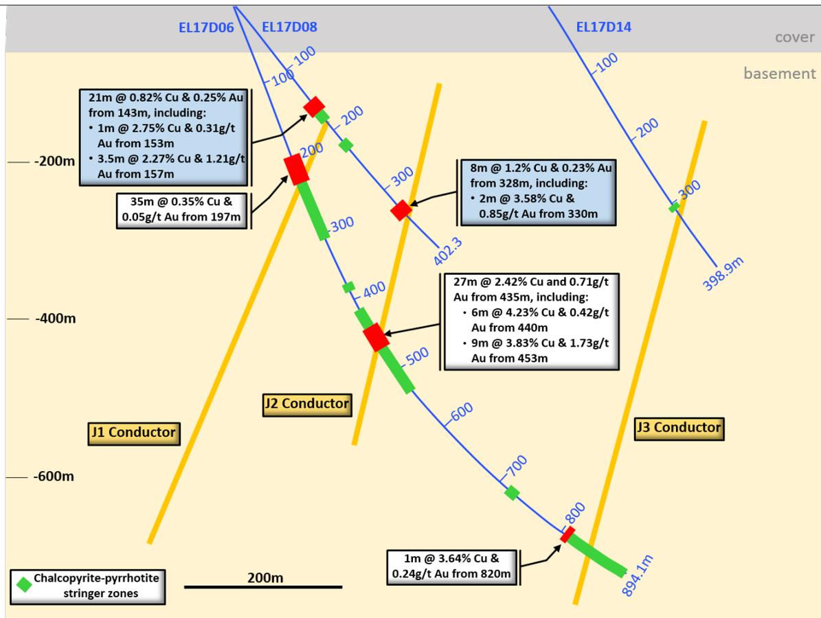
Figure 3: Cross-section (viewed north) at Jericho prospect showing completed drill holes EL17D06, EL17D08 and EL17D14, the 3 modelled EM plates and zones of copper mineralisation
