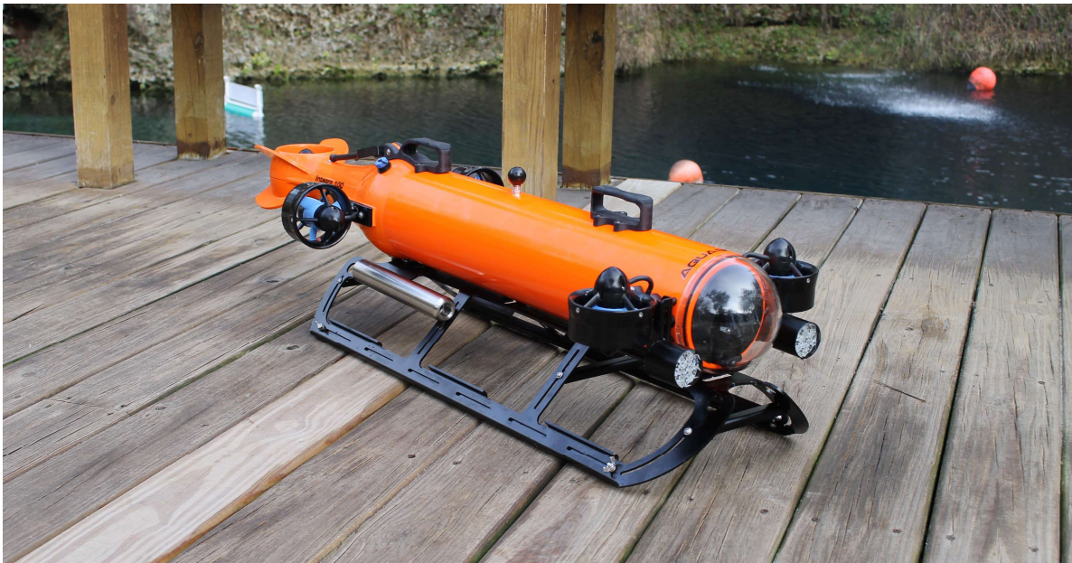
Aquabotix’s second-generation hybrid vehicle, the Integra AUV/ROV
