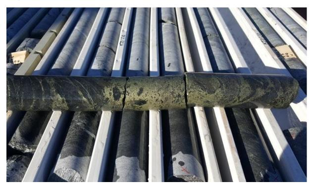
Photograph 1. KJD220W1 at Reward zone of massive sulphides at ~564m hole depth, corresponding to Conductor R1.
