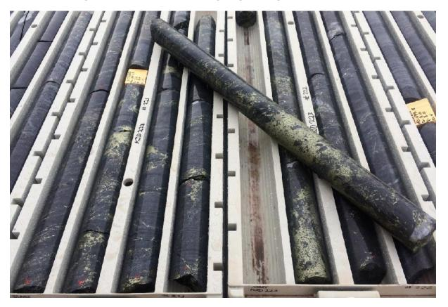
Photograph 2. KJD223 at Reward Prospect - Chalcopyrite in banded and brecciated magnetite circa. 692-698.5m, corresponding to Conductor R6.
