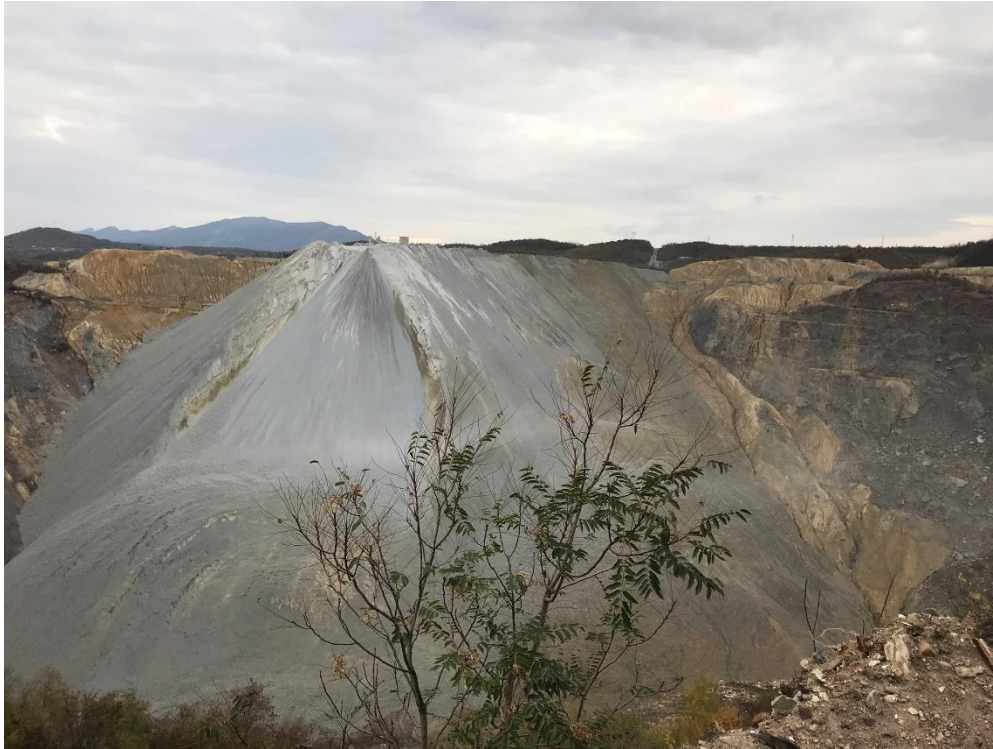
Figure 40. Bor Copper-Gold open-cut mine, actively back-filled with waste material.
