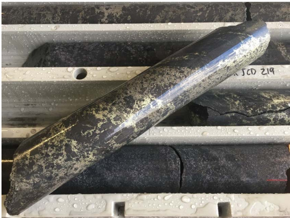
Photograph 2. Hole KJCD219 Magnetite breccia zone
