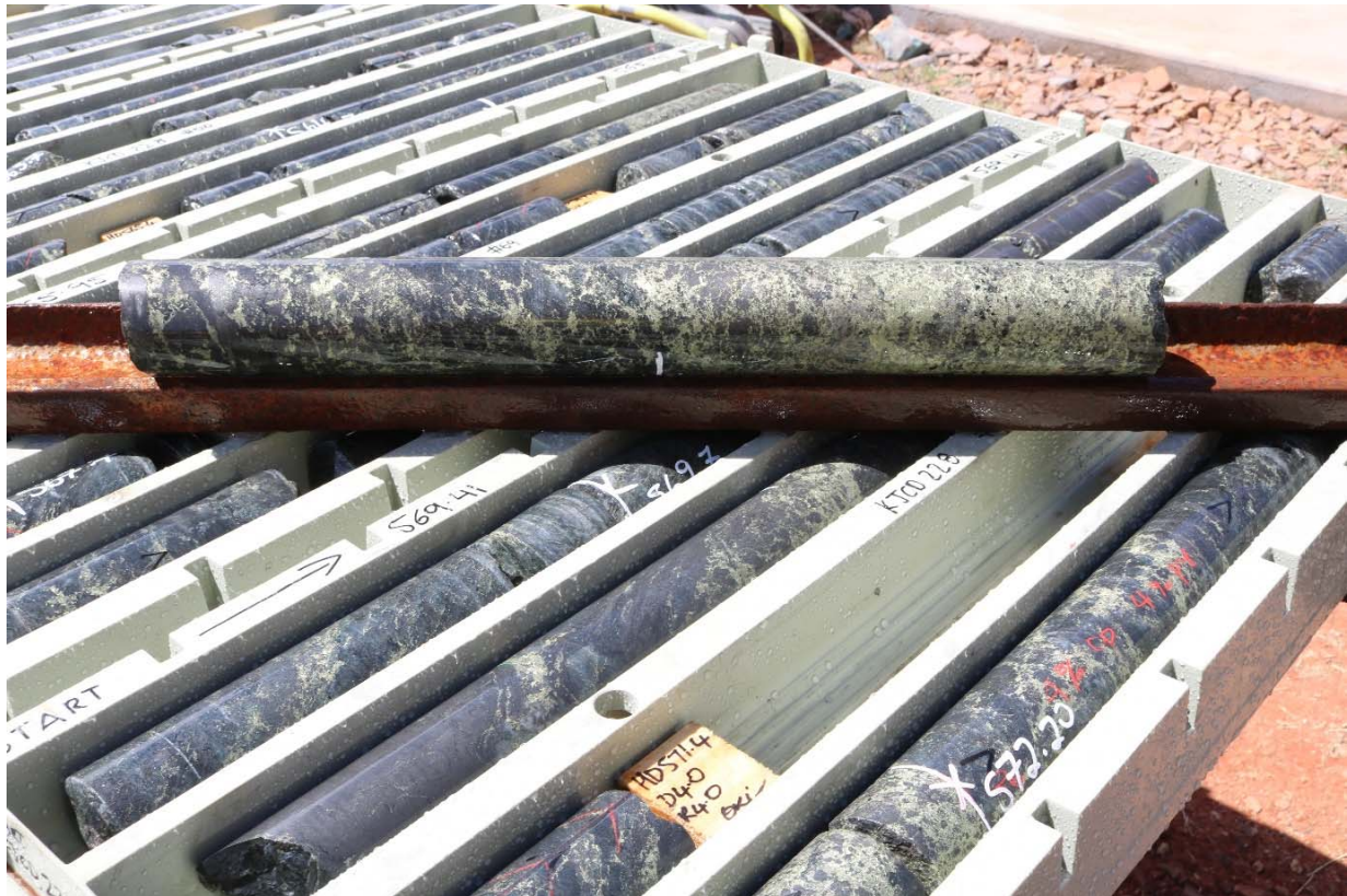
Photograph 8. Massive magnetite with breccia matrix of chalcopyrite, from 571.68 to 572.2m.
