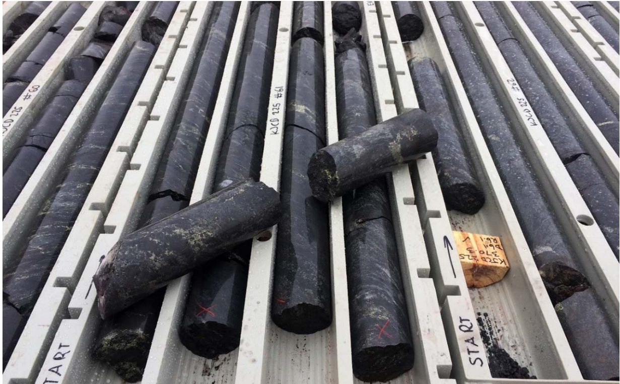
Photograph 5. KJCD225 Disseminated chalcopyrite in massive magnetite circa. 692-698.5m.
