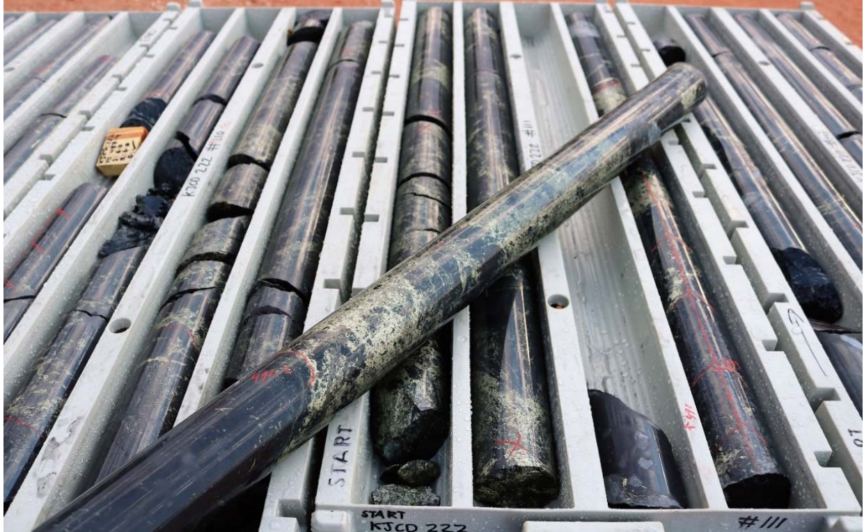
Photograph 4. KJCD222 Chalcopyrite-magnetite breccia circa. 492m, corresponding to Conductor C3
