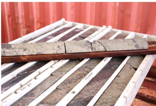
Photograph 6a. Massive sulphide zone showing a breccia matrix of chalcopyrite and pyrite
