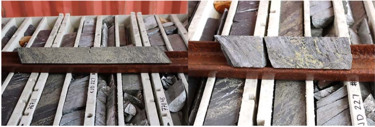
Photograph 7a. Massive sulphide and magnetite breccia (769.86 – 770.72 m).
