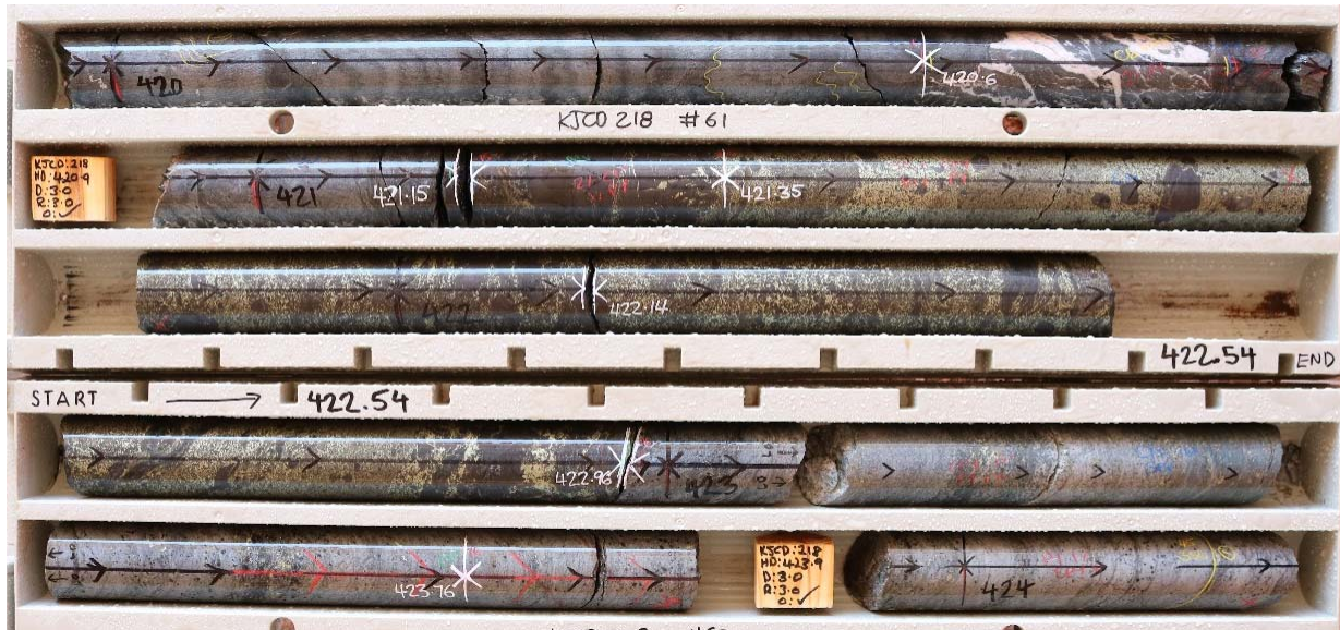
Photograph 1. Hole KJCD218 Zone of chalcopyrite dominated massive sulphide breccia matrix in massive magnetite host from 421.15 to 422.96m, corresponding to conductor C6.
