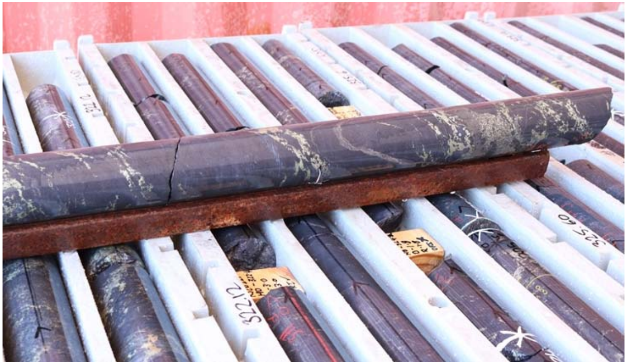
Photograph 3. KJCD221. Zone of massive magnetite vein with foliated sulphides from 308.5-325m, corresponding to Conductor C3.
