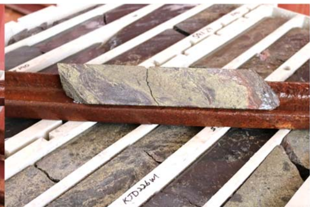
Photograph 6b. Pervasive vein-hosted sulphides within pelitic host unit.
