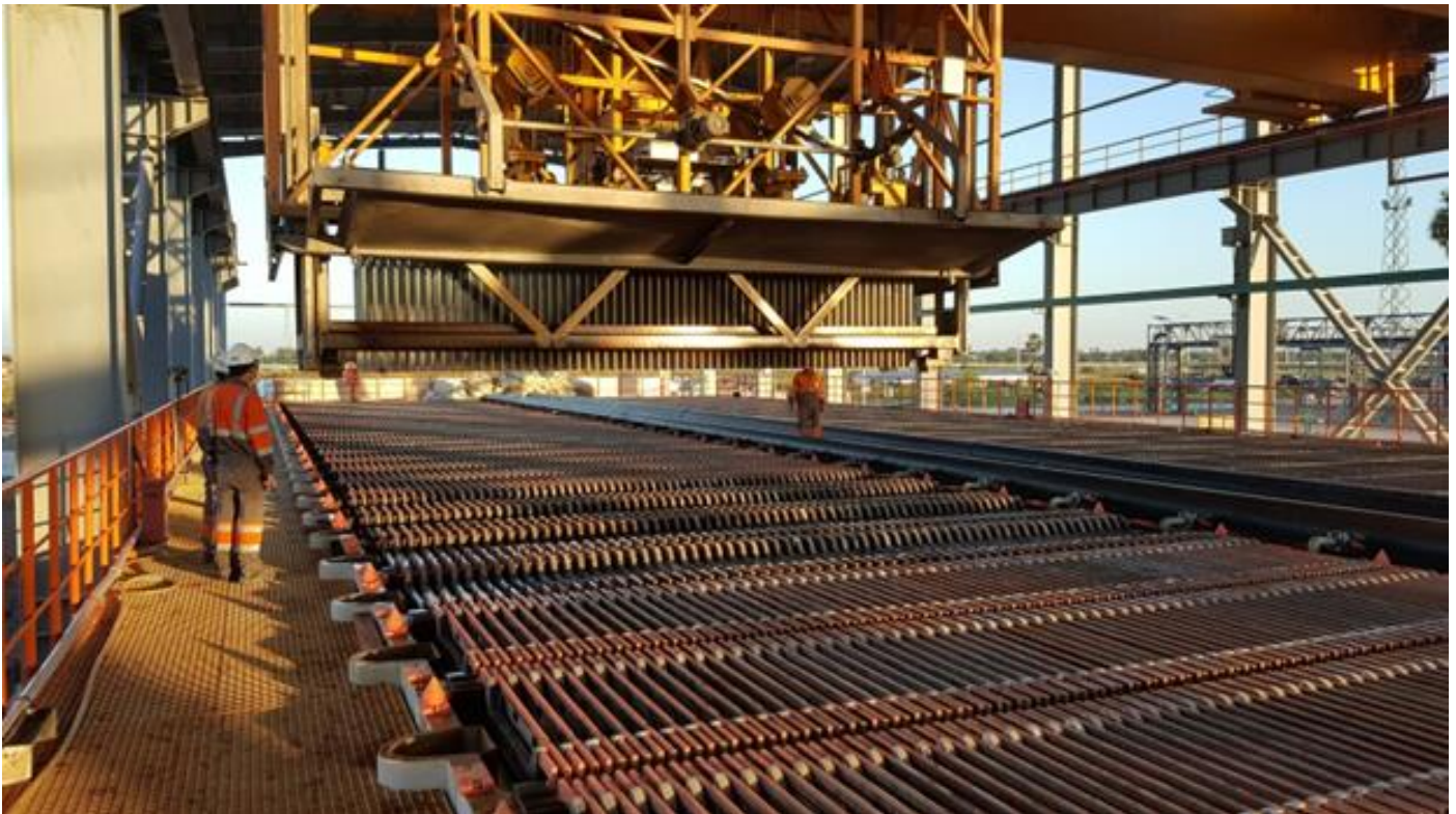
Electrowinning cells and copper cathode production at one of Wanbao Mining's operations in Myanmar.
