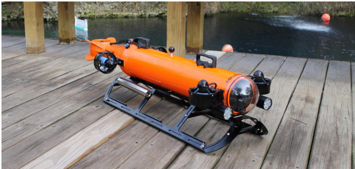
Aquabotix's second-generation hybrid vehicle, the Integra AUV/ROV
