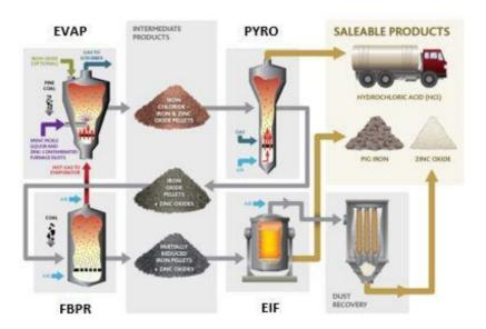
Each stage of the testwork program will process all the furnace dusts and SPL supplied by local steel makers in a simulated continuous campaign. The first three process steps are being undertaken at the Newcastle plant using both modified existing equipment and new purpose-designed equipment.
