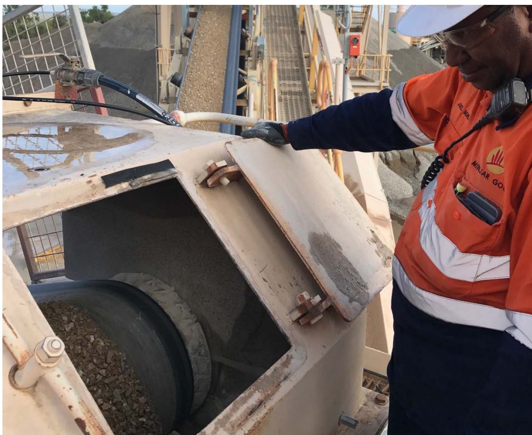
Figure 10: Belt sampling of Piccadilly ore occurring at Pajingo Mill
