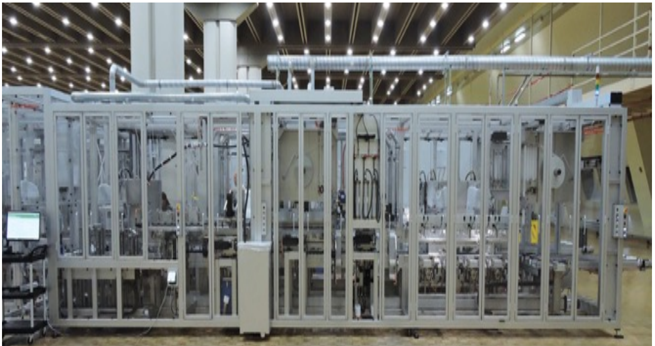
Figure 3 - Electrode Stacking Equipment
