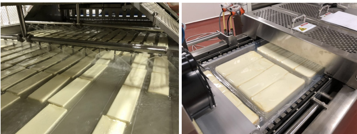
Photos above of the mozzarella in the brine and being sealed into individual blocks.
