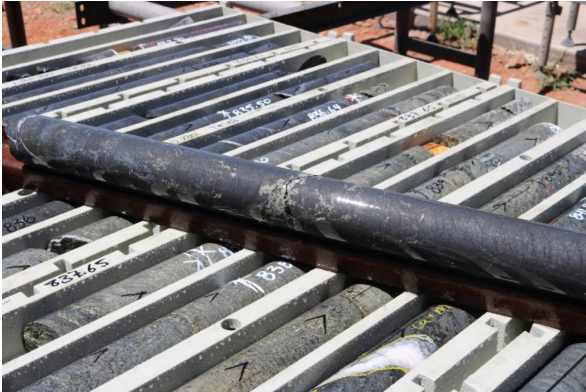
Photograph 1. Hole KJCD230 - Zone of massive magnetite with disseminated chalcopyrite and pyrite stringers (Conductor C8) circa 831.5m.
