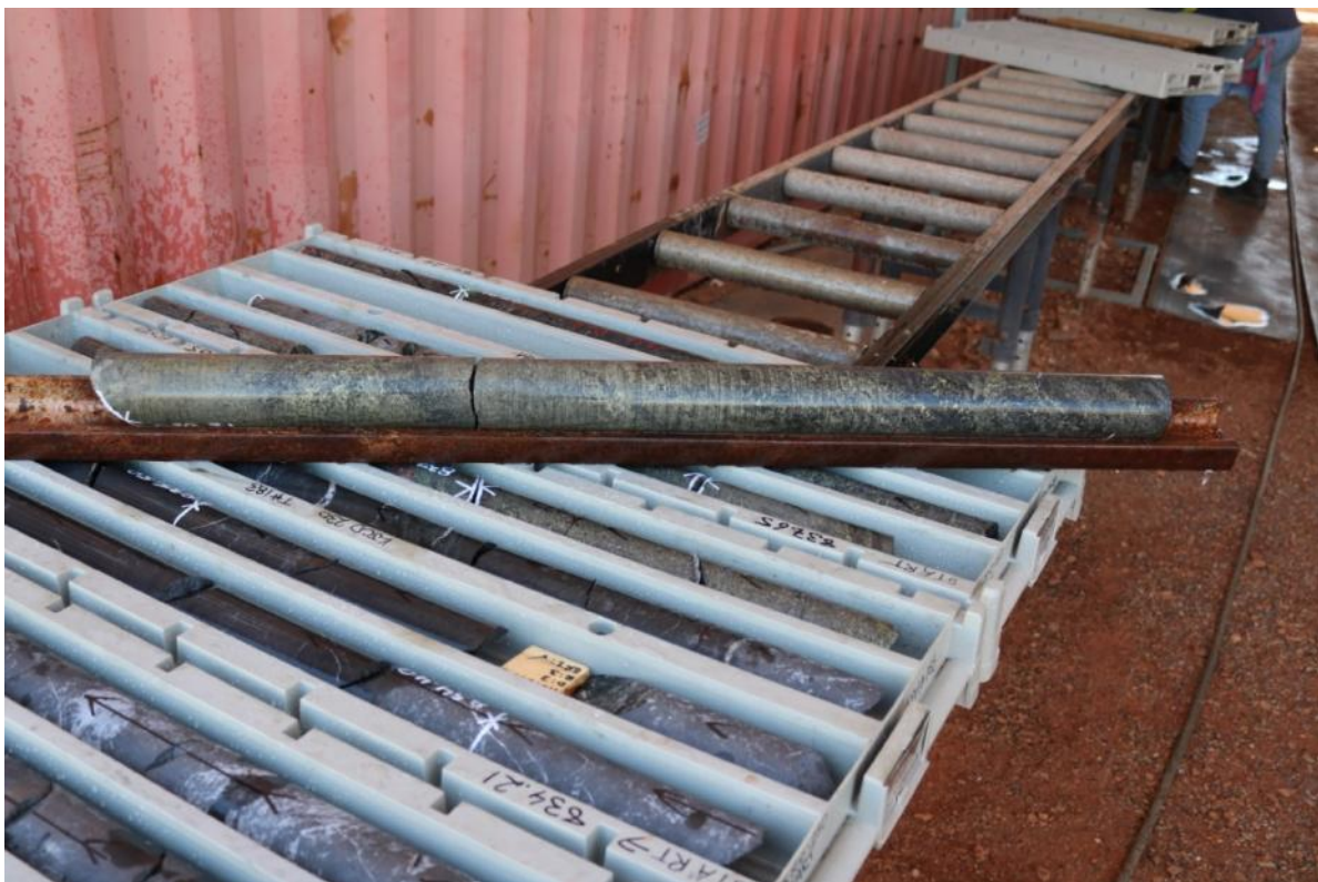
Photograph 2. Hole KJCD230 - Zone of disseminated breccia matrix sulphides chalcopyrite and pyrite with magnetite vein (Conductor C8) circa 839.31 m.
