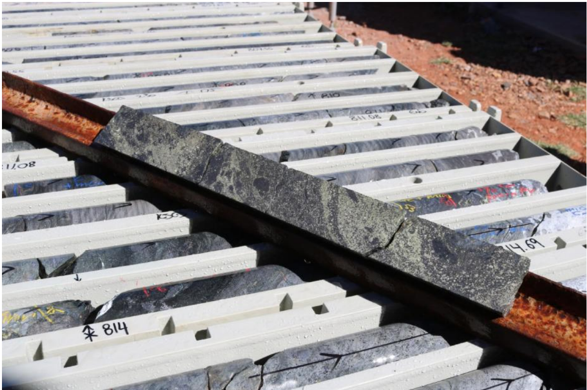
Photograph 4. Hole KJCD234 - Zone of semi-massive and foliation-controlled chalcopyrite, with brecciated magnetite (Conductor R1) circa 279.04m.
