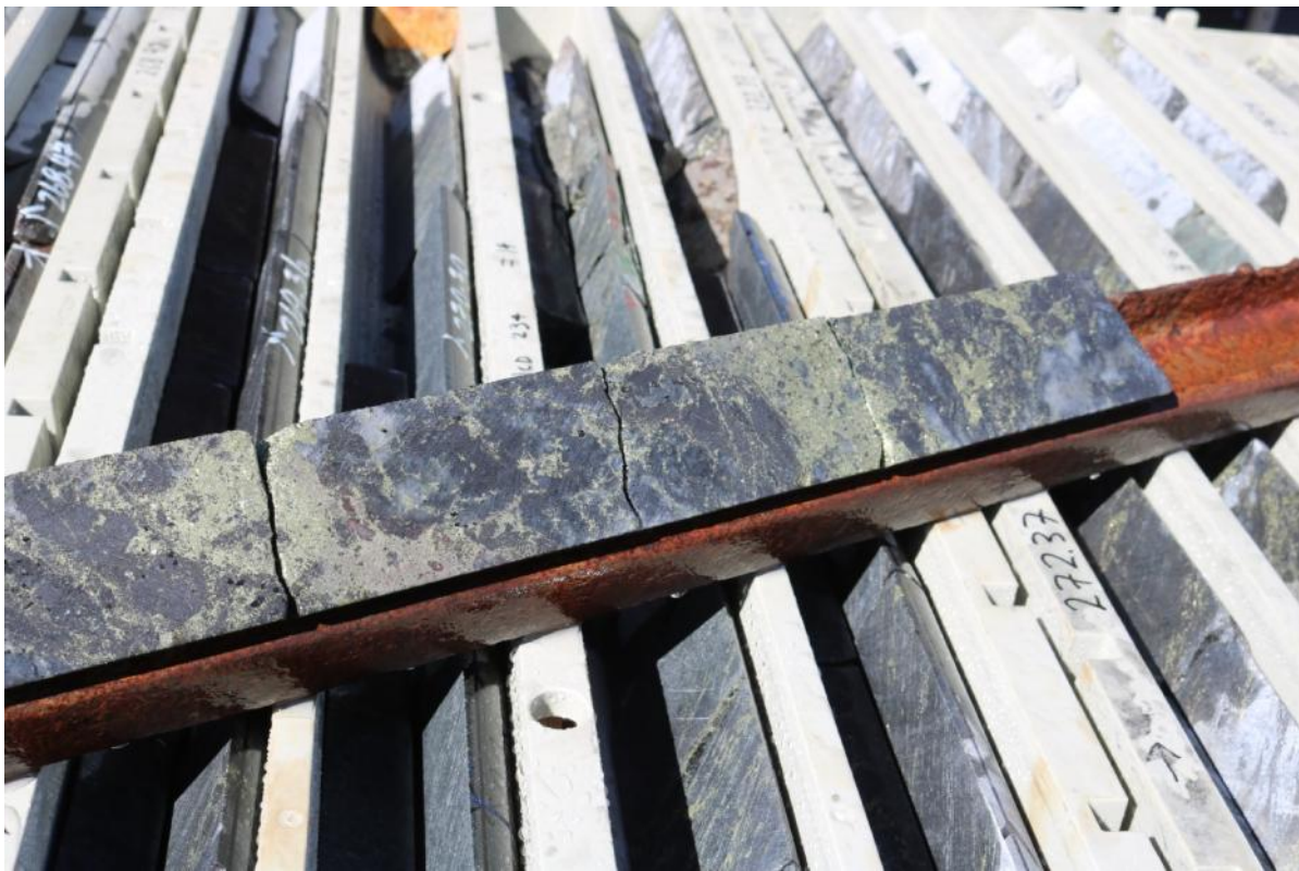
Photograph 3. Hole KJCD234 - Zone of semi-massive chalcopyrite and breccia of magnetite (Conductor R1) circa 275.13m.
