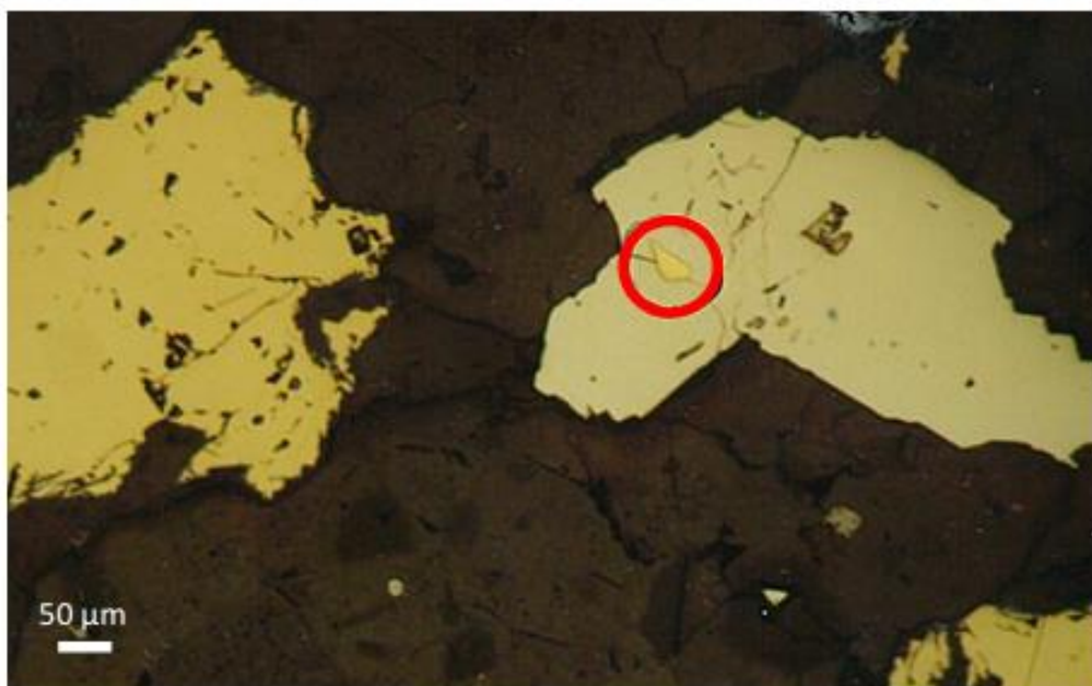
Figure 13: Photomicrograph from Walparuta Cu-Au Mine. Yellow Mineral = Chalcopryite, White Mineral = Pyrite and Red Circle = Au (25x50μm) (Pontifex, 1990).
