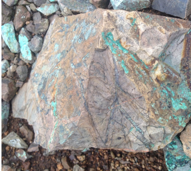
Example of copper mineralisation at surface on the Canhada Target. Hydrothermally altered volcanic rock with malachite filling fractures in stockwork pattern. Sample grading 4.09% Cu
