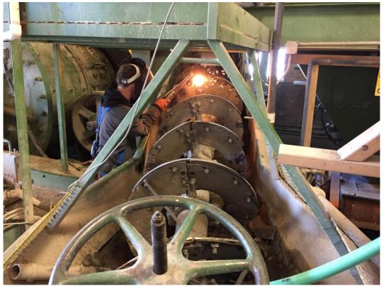
Image 4: Cutting old bolts to replace classifier blades
