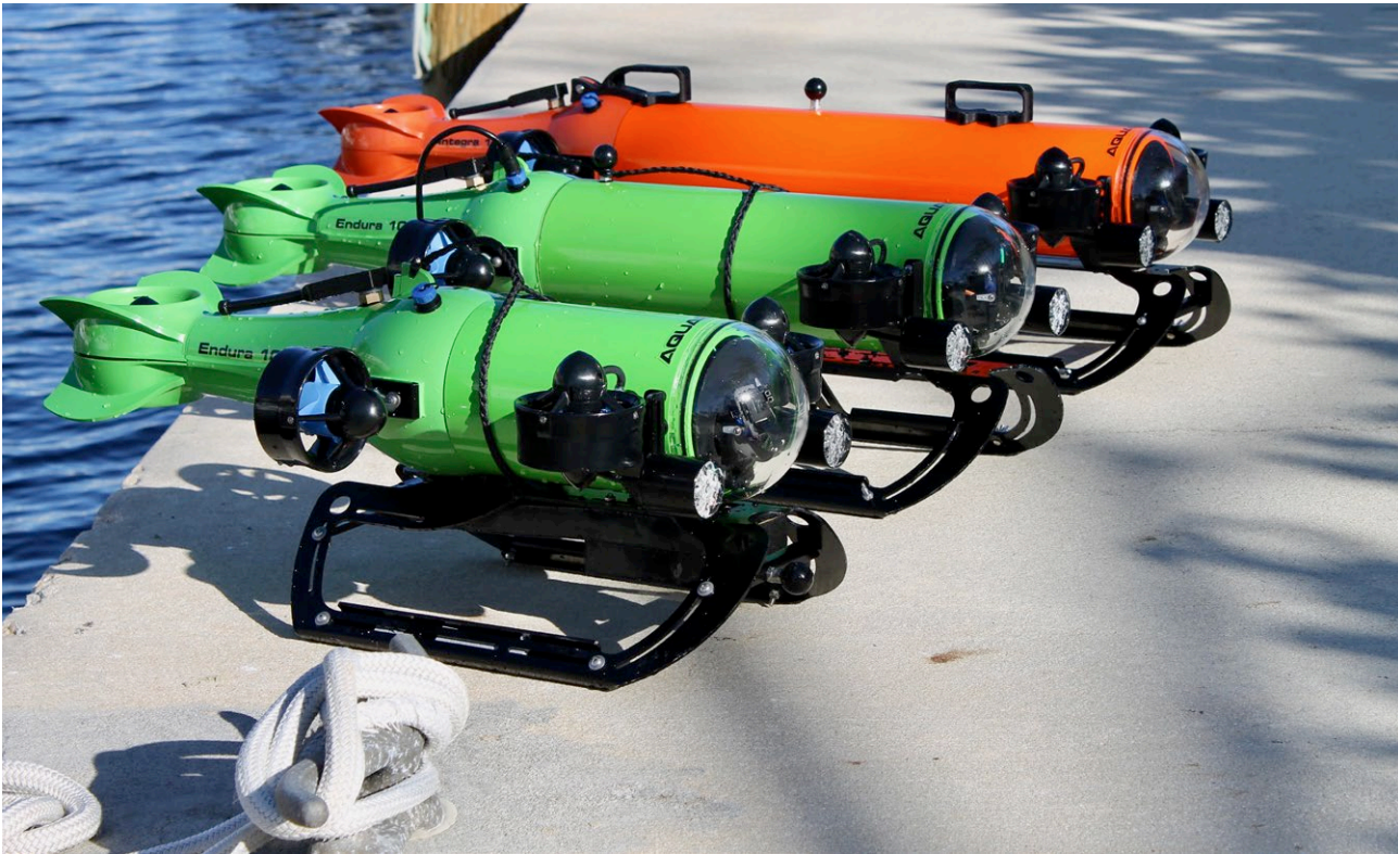
Image above: Endura and Integra underwater vehicles with varying body lengths, to accommodate differing payloads.
