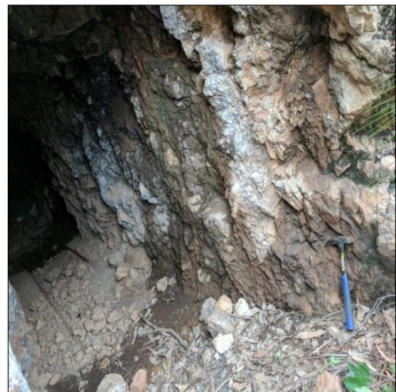
Figure 1b – Target zone weathered serpentinite (above & left of hammer)
