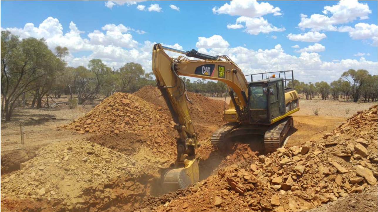
FIGURE: Excavation of bulk phosphate rock sample for crusher test work at Ardmore.
