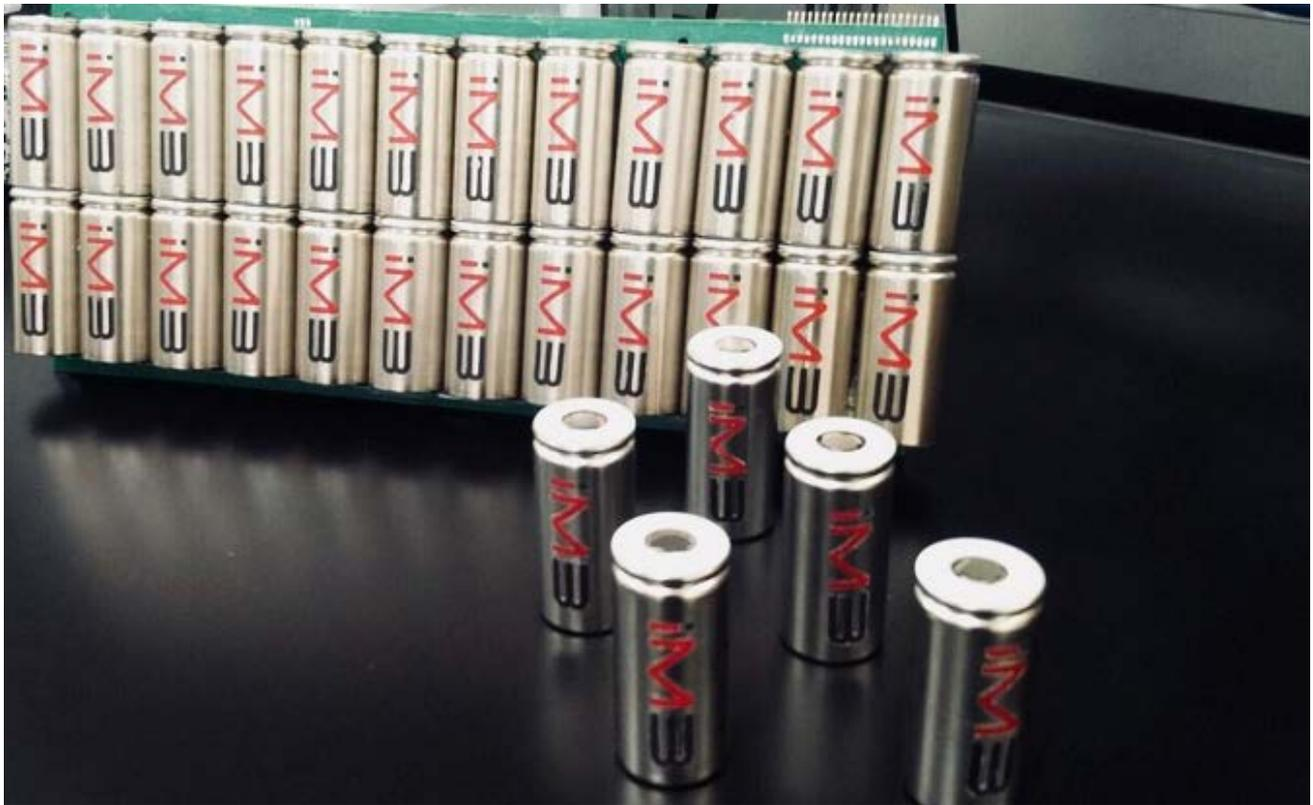
Figure 1 – Cylindrical cells produced by Magnis part-owned consortium using B&W MEGTEC coating lines
