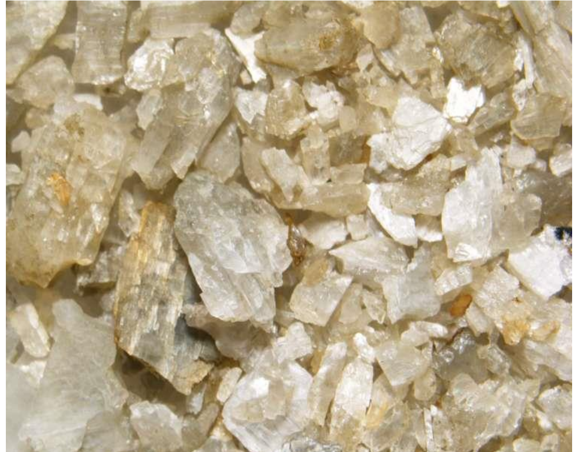
8.10% Li 2 O Spodumene from HLS Testwork
