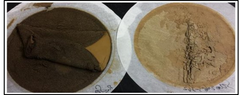
Pilot plant testing at Eriez using a rougher-cleaner flotation circuit. Difference in colour of the tails on the left and the concentrate on the right demonstrate the effect of the cleaner stage
