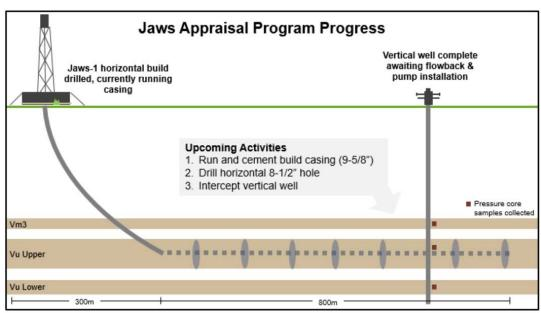
The Jaws-1 Project wells are being drilled by Halliburton in collaboration with Ensign on the 965. The horizontal well is the second of the two well appraisal campaign designed to prove commercial flow rates of gas and assess the quality of Strike's Southern Cooper Basin Gas Project (**SCBGP**) in PEL96 (Strike 66.67% and Operator, Energy World Corporation 33.33%).
