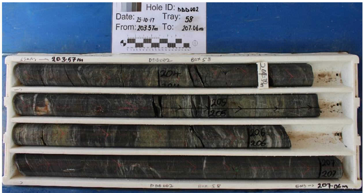
Figure 7: DDD 002 – Intense quartz-carbonate veining, part of interval 203-206m, 3m averaging 1.10 g/t Au
