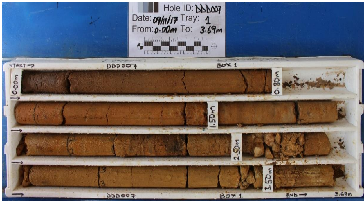
Figure 4: DDD 007 – Weathered Saprolite core with broken quartz veining, interval 2-3m, 1m averaging 8.09 g/t Au
