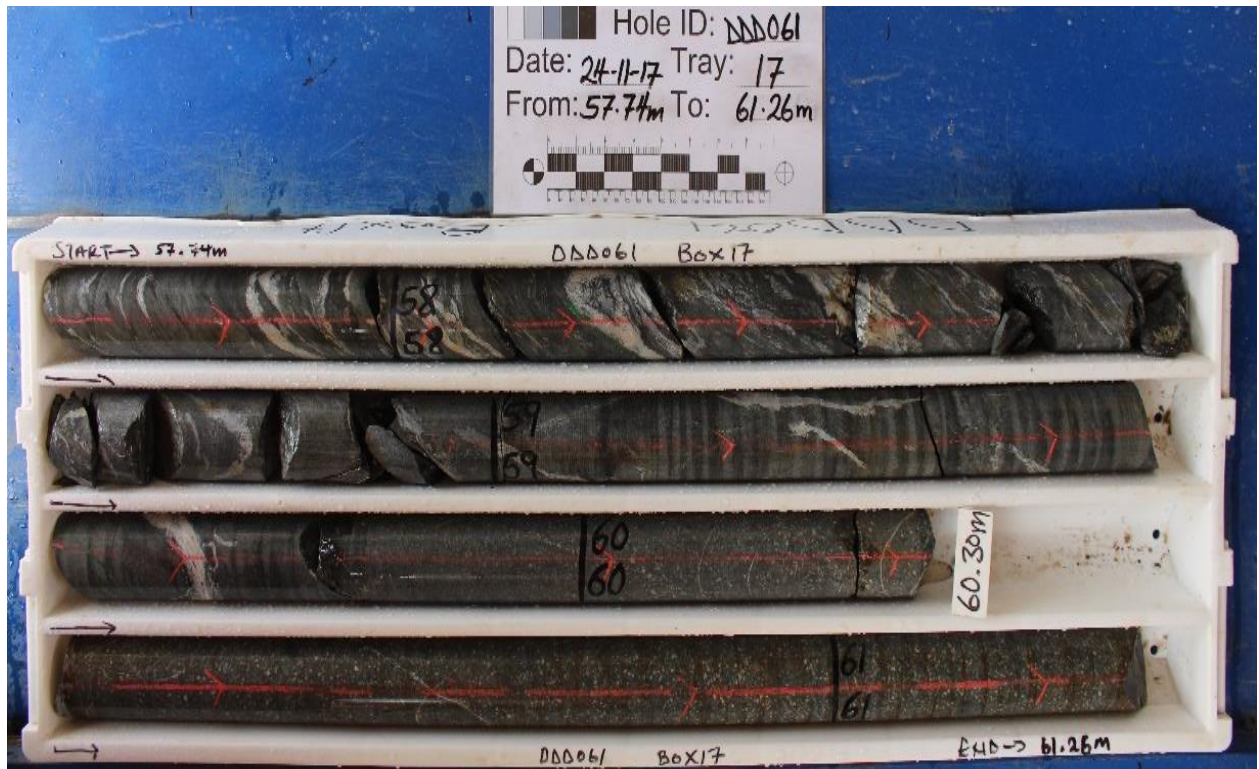
Figure 6: DDD 061 - Intense quartz-carbonate veining, interval 57.8-60m, 2.2m averaging 2.21 g/t Au
