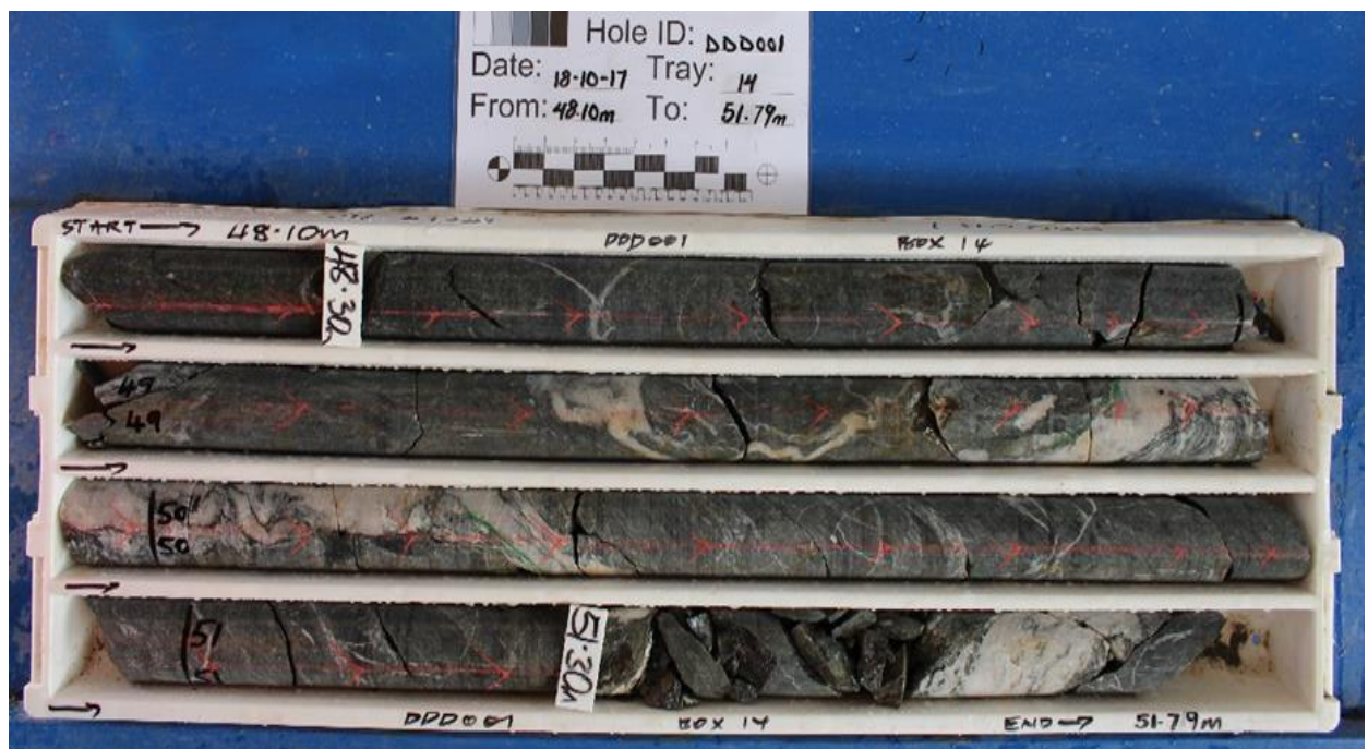
Figure 5: DDD 001 – Intense quartz-carbonate veining, part of interval 48-52.5m, 4.5m averaging 1.03 g/t Au
