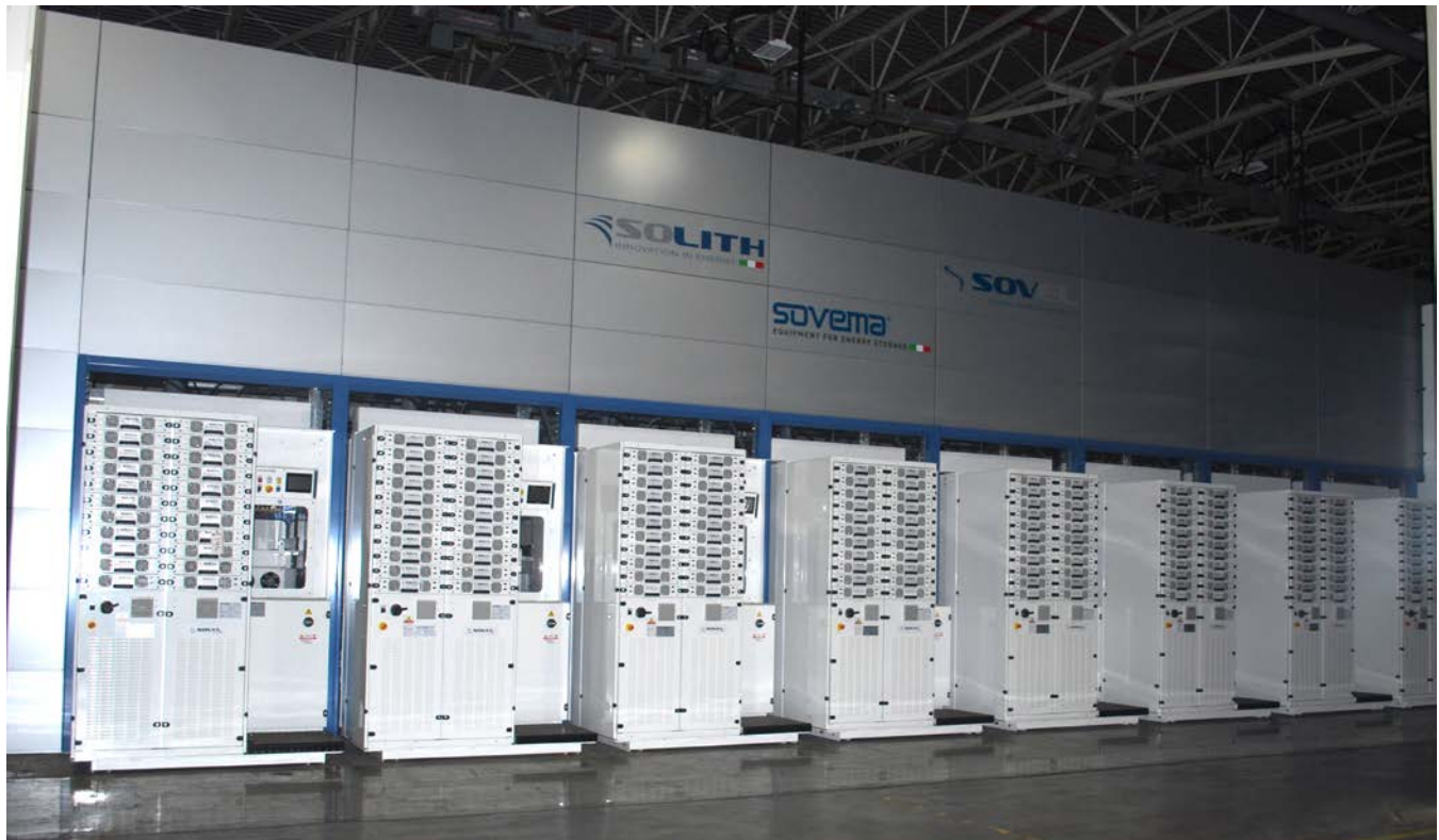
Figure 4: Portion of fully robotized formation equipment
