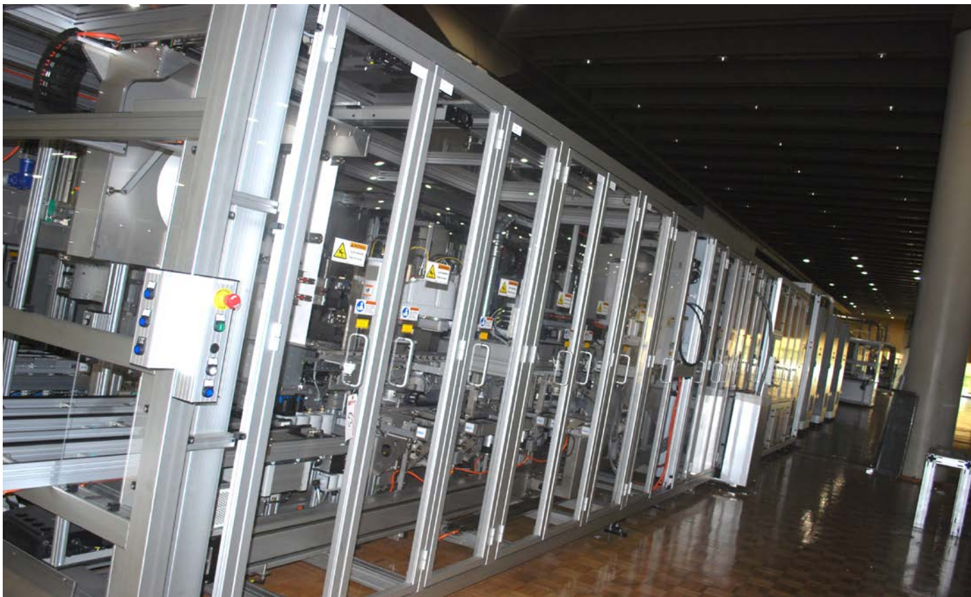
Figure 2: Portion of iM3NY's fully automated cell assembly line
