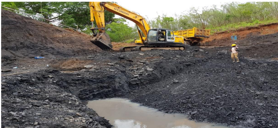
Exposing Coal seam in the Northern Pit from the outcrop
