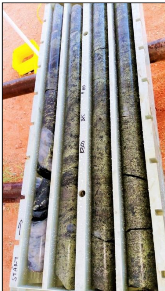
Photograph 1: Massive sulphide/magnetite breccia ~579-583 m (Conductor 6)
