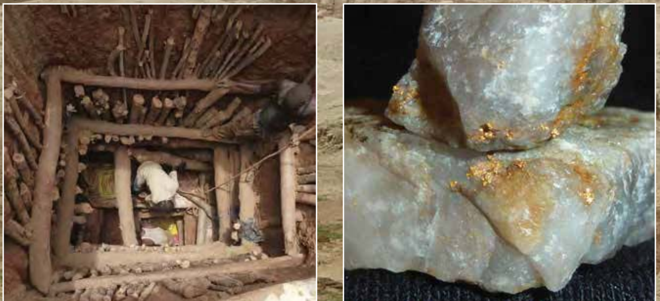
FIGURE 4.10 Niou Artisanal Site; right image is gold in quartz veins from this site; left image is one of the many artisanal mine shafts
