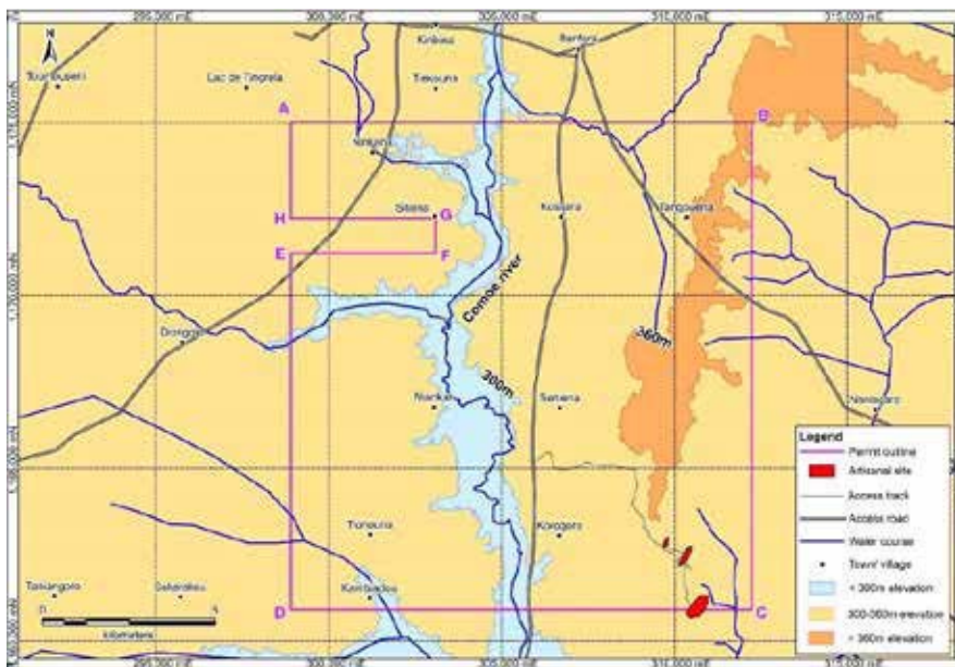
Figure 32: Simplified topography within the Tangora Permit with streams, tracks and the area of main artisanal mining (red circle). UTM (WGS84z30N)
