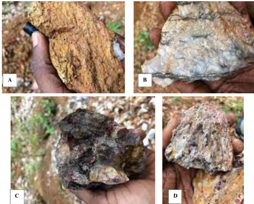
Plate 6: Rock chip samples collected from artisanal workings within the Tchaga soil anomaly: A) weathered sediment with traces of pyrite & carbonate alteration, B) quartz vein with carbonate C) sediment / quartz vein contact zone with manganese D) strongly weathered and sheared sediment from artisanal pit: 228,218E / 1,015,991N UTM (WGS84z30N)
