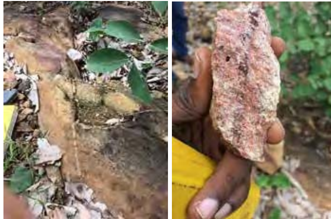
Plate 7: Tchaga prospect, granite outcrop cross cut by narrow (1cm) quartz veins oriented 080° and dipping 80° degrees to the south, 228,302 / 1,016,164 UTM (WGS84z30N)
