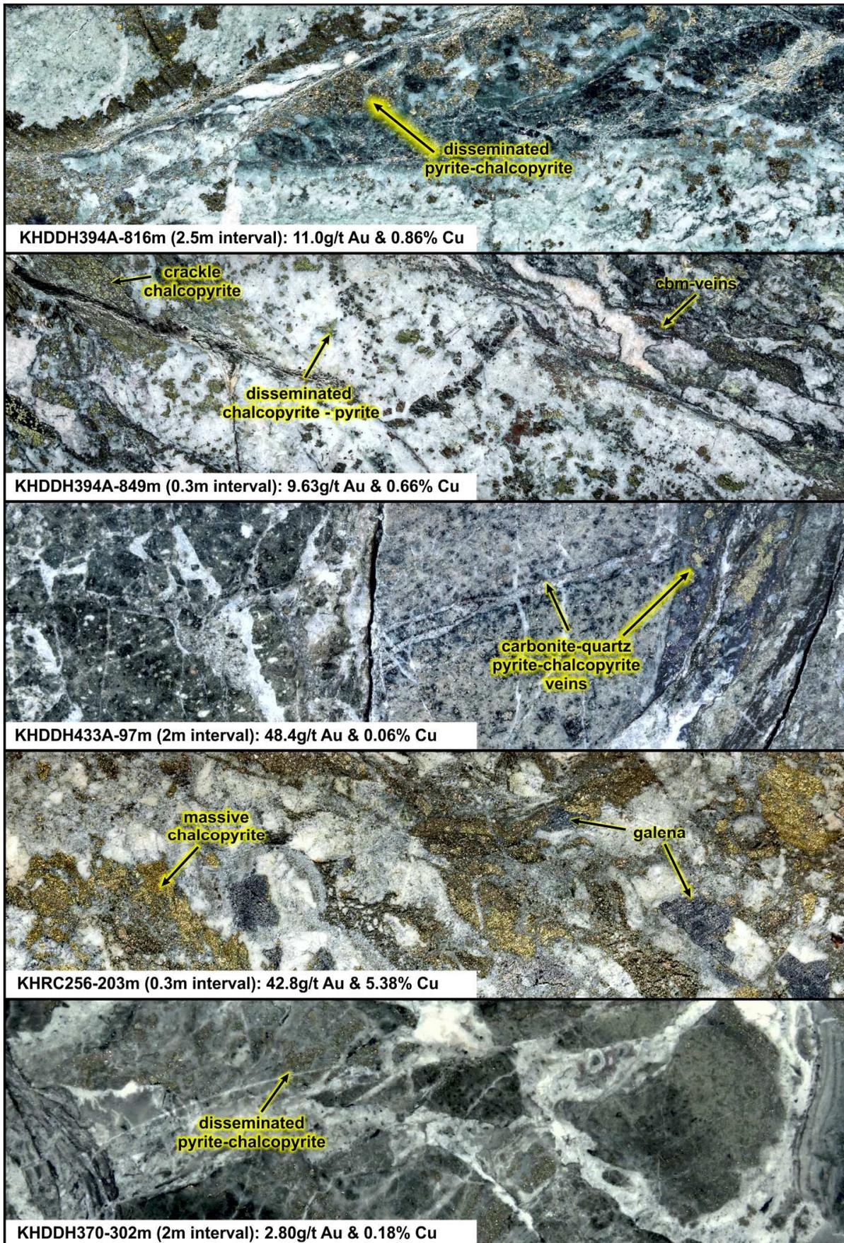
**FIGURE 8:** A selection of historic epithermal gold intercepts from Kharmagtai. Halved HQ core, the height of each image is 6.35cm.
