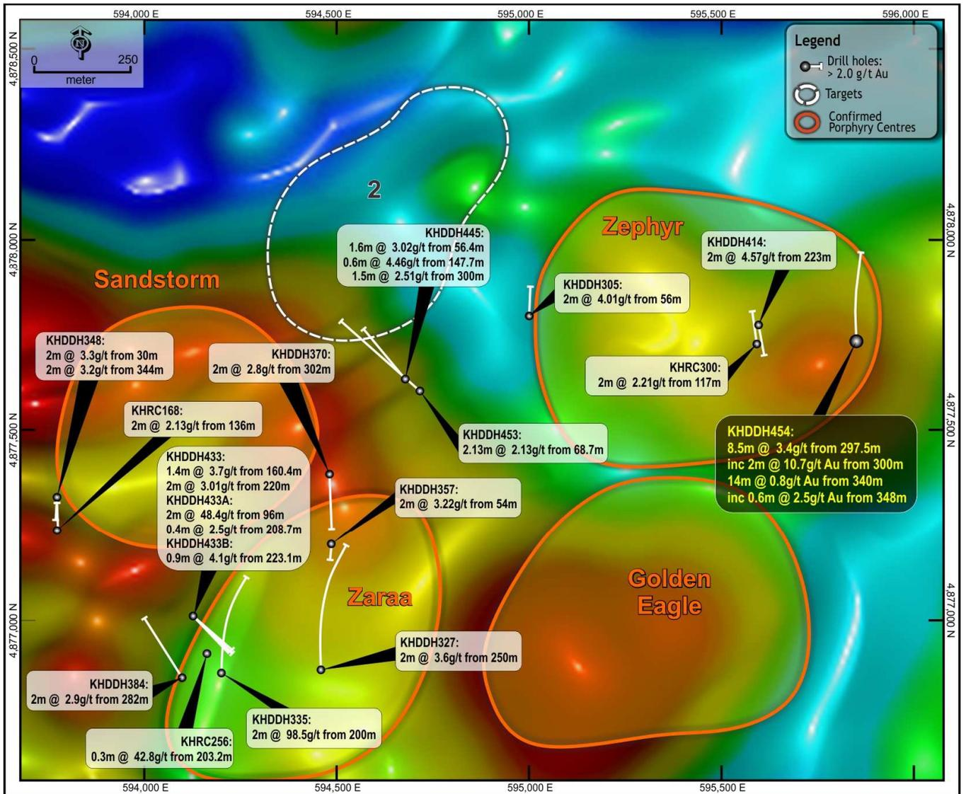
FIGURE 7: Plan showing the location of KHDDH454, intercepts and historic epithermal intersections over 2g/t Au.
