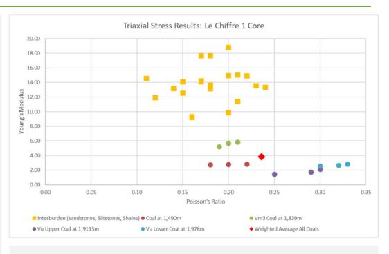
(above) A plot of triaxial stress tests from the coals and interburden in the Le Chiffre cores. These indicate the appropriate conditions for implementing IVFC are met through the relationship of the interburden and Vu Upper coal.
