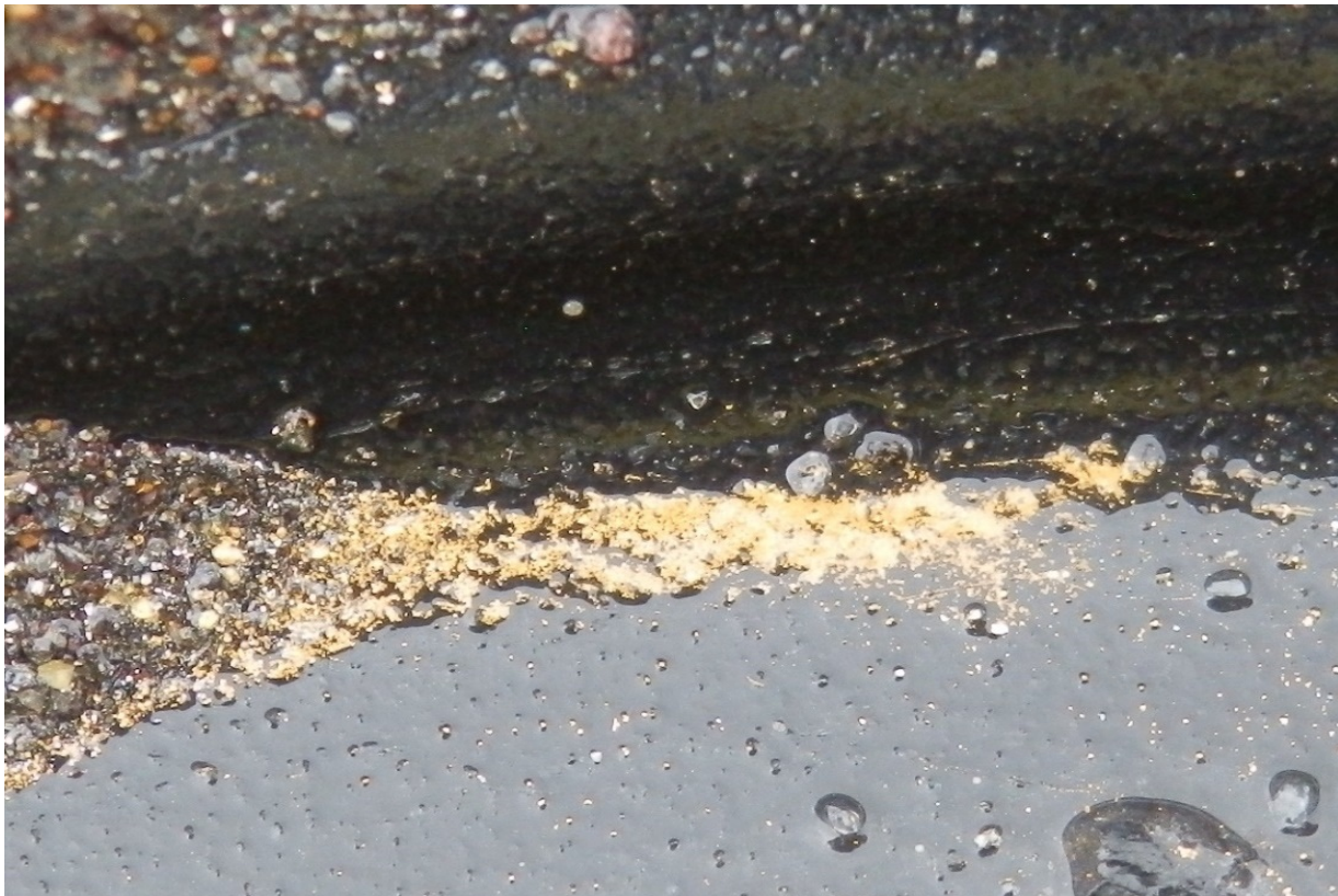
Figure 7: Close up of visible Au tail in panned concentrate from crushed Piccadilly lode.
