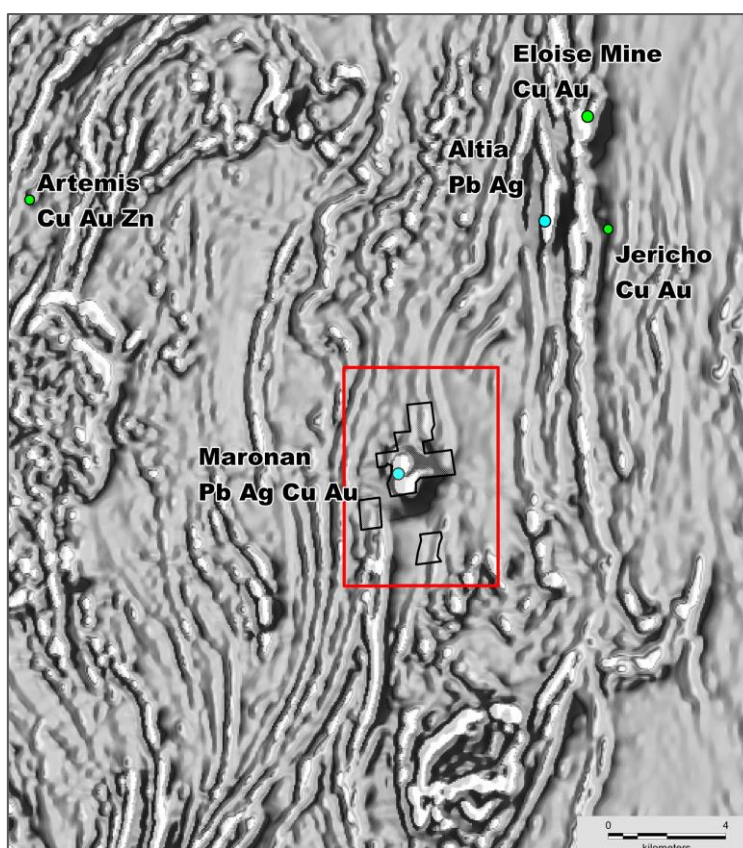
[Figure 1] Maronan Project: Regional vertical gradient magnetic image showing the Maronan lead-silver and copper-gold deposit, other copper-gold and lead-silver-zinc prospects and the Eloise mine. Historic ground electromagnetic survey grids on Maronan are shown as black polygons.
