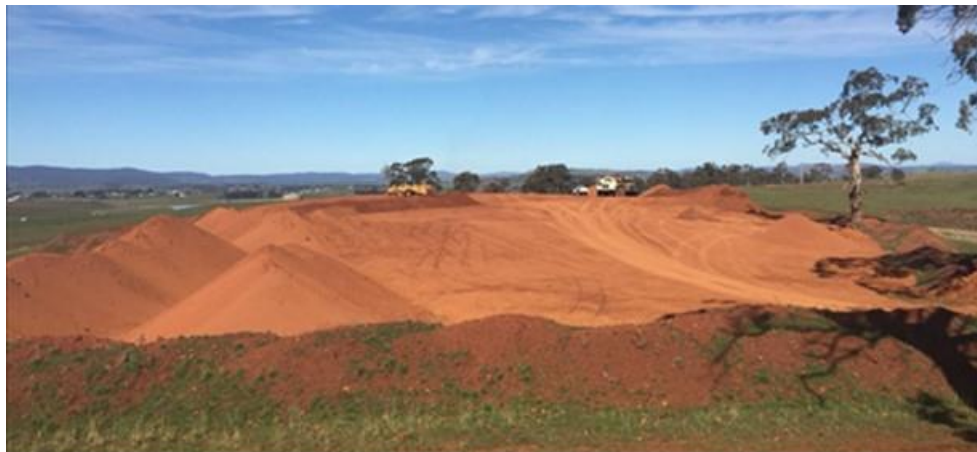
Figure 3 End of mining January 2016 Topsoil was stored in bunds around the mining areas and kept “alive” by not burying it in large stockpiles.
