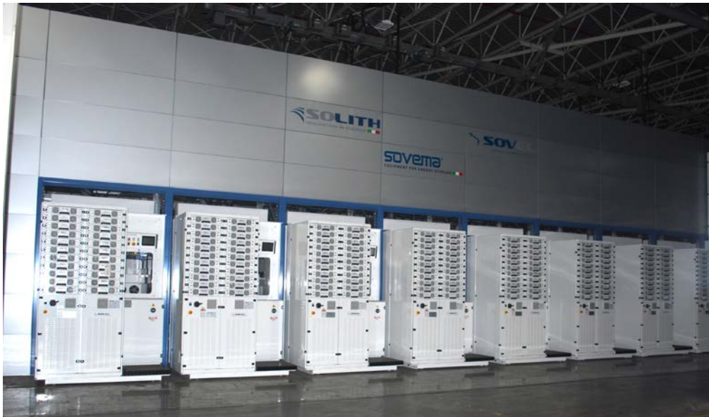
Figure 2: Portion of fully robotized formation equipment
