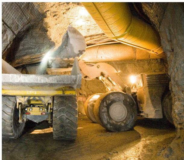
Underground during trial mining loading rock into truck for haulage to the surface. This was at the 'Warrior' mine, located about 5 kilometres from 'Central'. Future mining will be at 'Central' where there are many more reefs.
