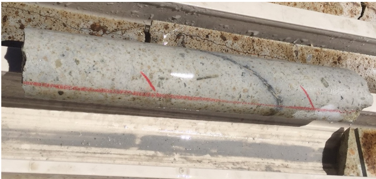
Figure 2. Porphyritic felsic intrusion in drill hole BRD17095.
