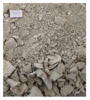
Sample before column leach test Lightly crushed to minus 150mm Coarse material with low % of fines
