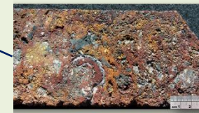
Iron/manganese altered polymict breccia at dolomite interface
