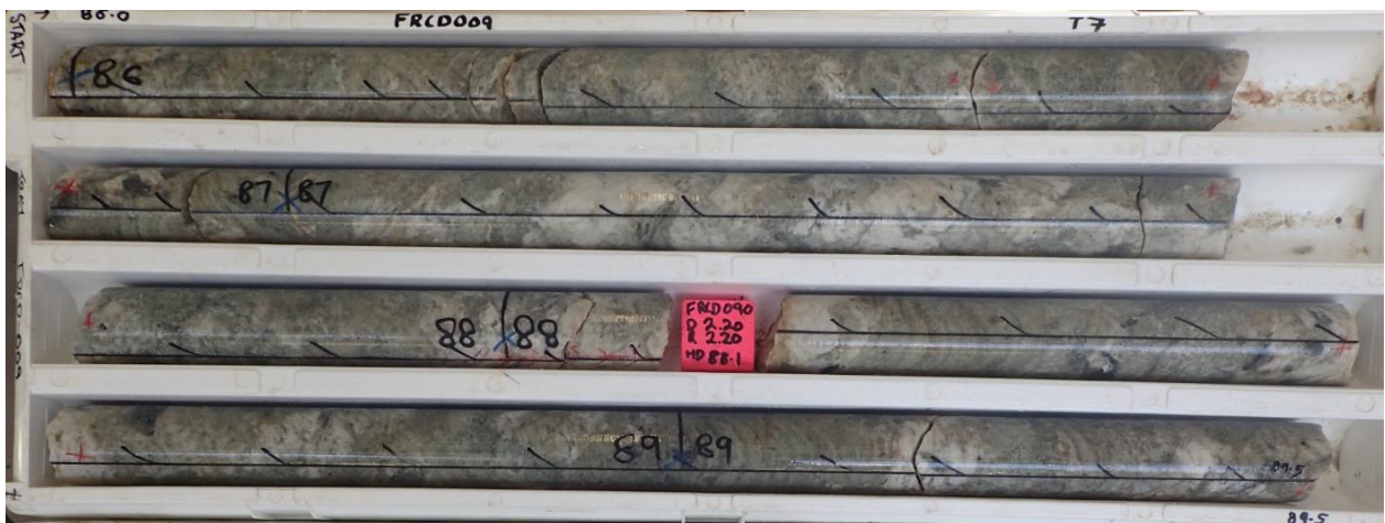
Figure 2 – Example of spodumene rich pegmatite drill core from Grants
