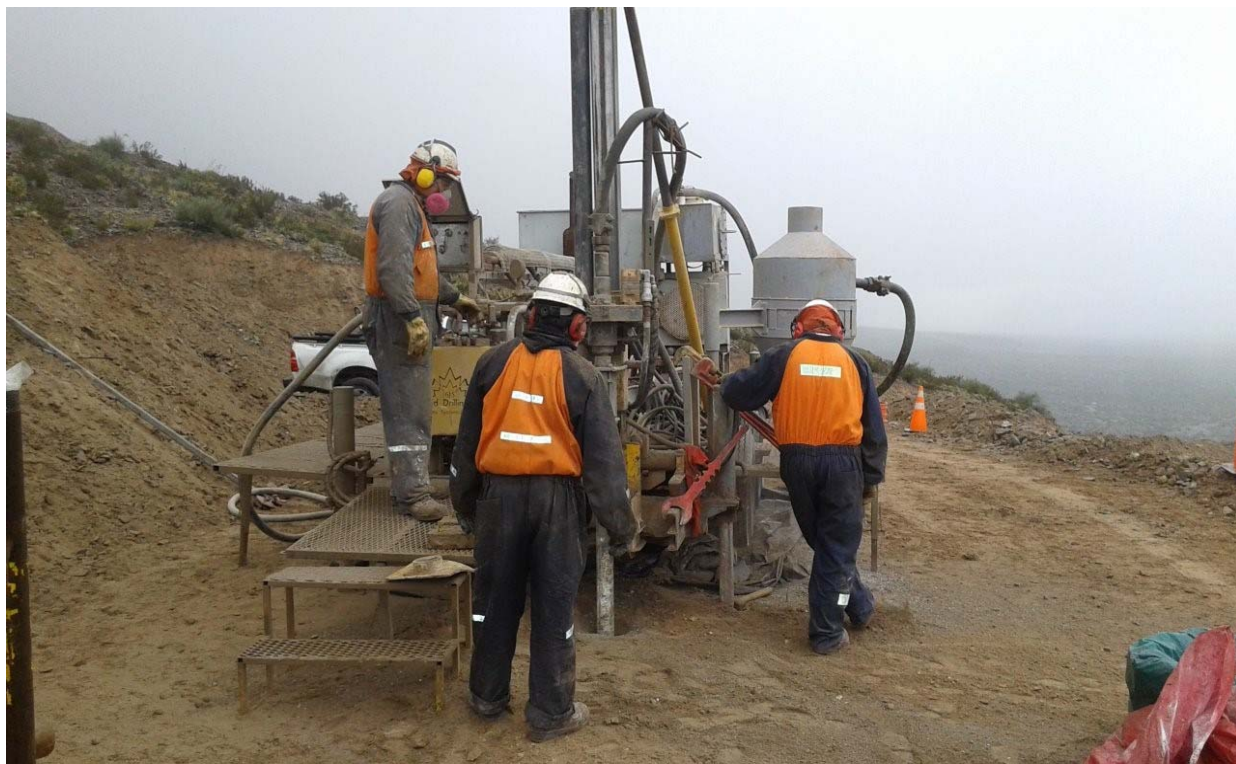
Photograph 2: The Energold Argentina SA diamond core drilling rig to be used at Las Tapias.
