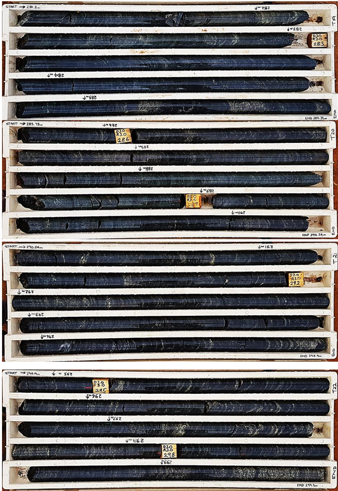
Plate 2 Example of the style of mineralisation encountered in intersections from the North Zone. This example is from hole 18CB057: 268 -299m. Black rock is magnetite. Fine yellow-bronze speckle and stripes throughout the rock is a predominantly chalcopyrite
