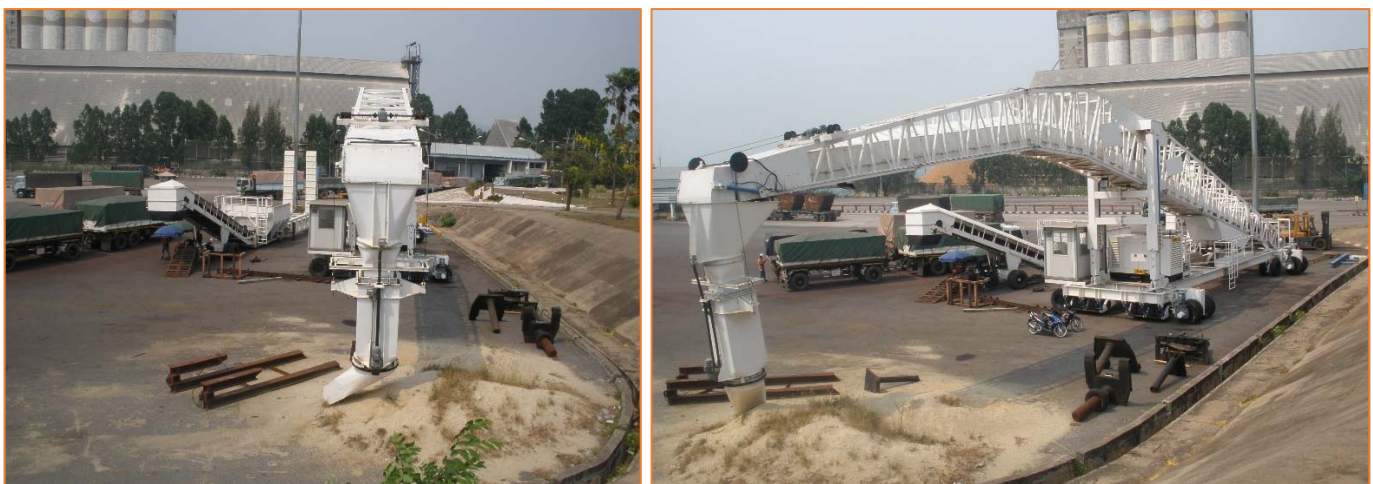
Above – photos of recently purchased 500tph ship loader and feed preparation conveyor system that will be transported to PNG
