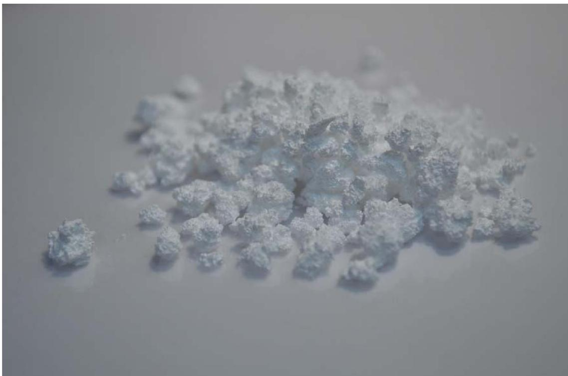
*High Purity Alumina crystals (99.9855% Al<sub>2</sub>O<sub>3</sub>)*
