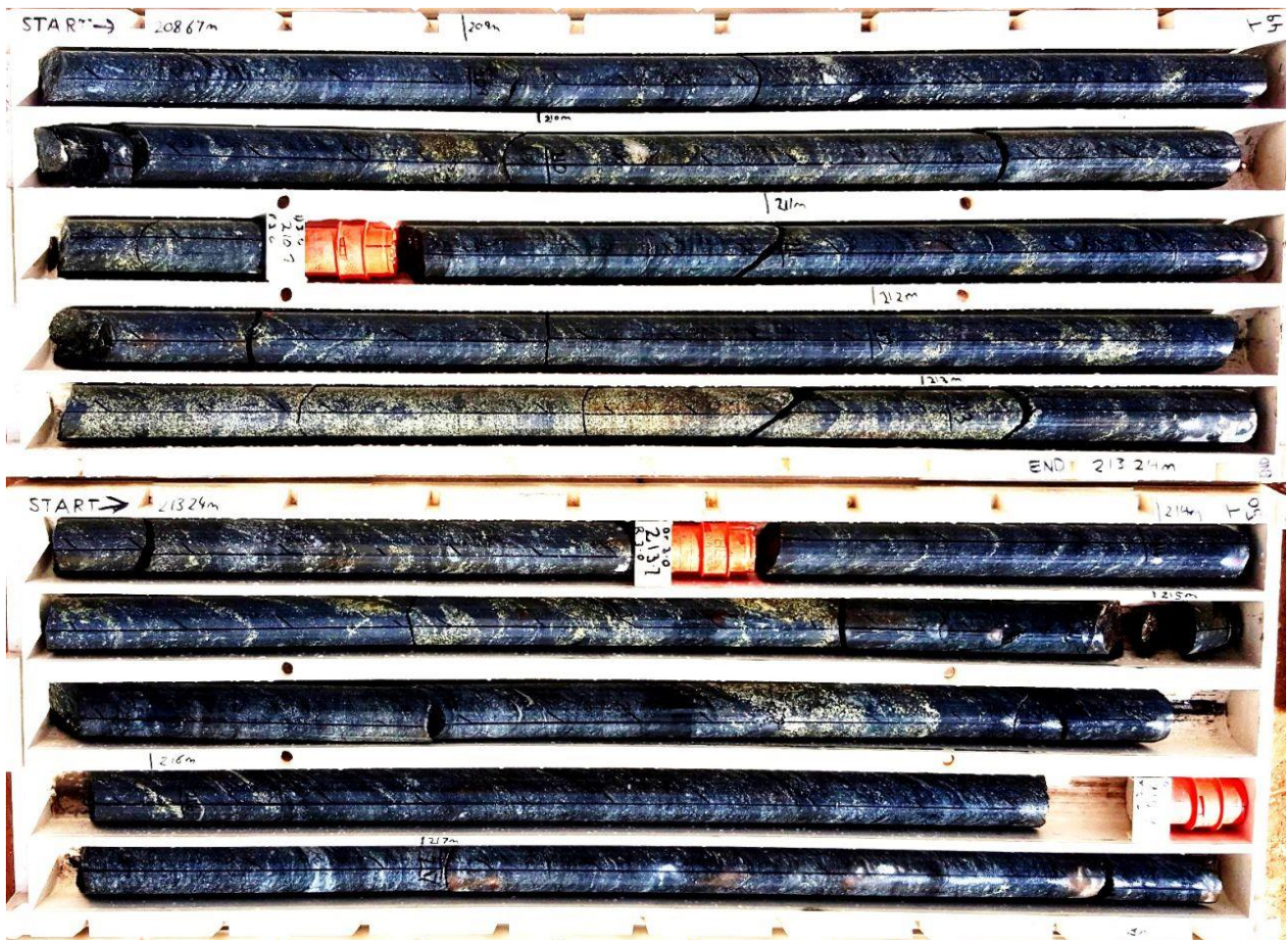
Plate 1 Example of abundant copper mineralisation in magnetite rich rocks in hole 18CB054. Black is predominantly magnetite, biotite and quartz. Yellow-bronze speckle is sulphide dominated by chalcopyrite (copper sulphide). The IP survey responds well to this style of mineralisation. (see Figures 1-3).
