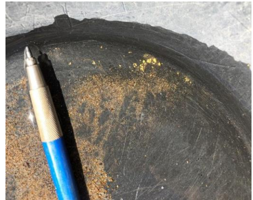
Figure 1: Photo of coarse free gold panned from TFRC011, 21 to 24m, Gallon Prospect.
