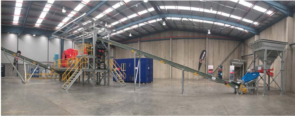
Figure 3: TOMRA 1200 XRT Ore Sorter and ancillary equipment
