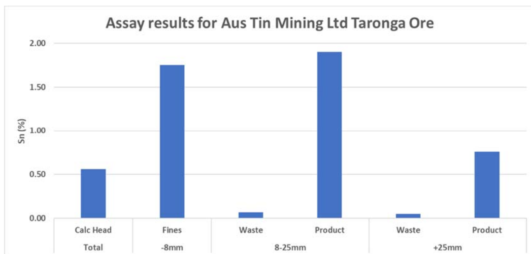
Figure 1: Assay results for sorted and unsorted fractions using TOMRA contrast-XRT (graph provided by TOMRA)
