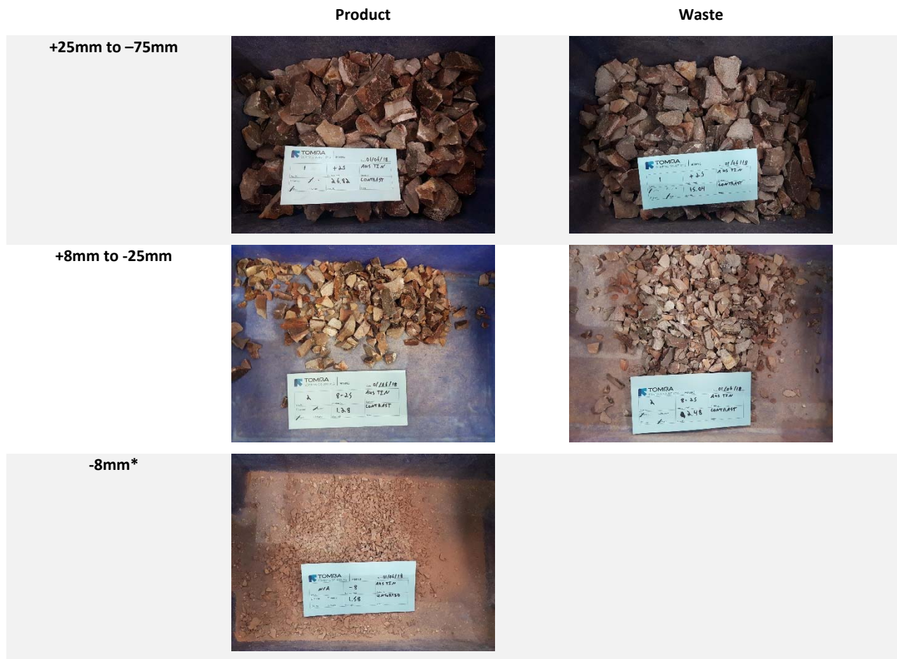
Figure 5: Images of Product and Waste streams generated using contracts XRT ore sorting
