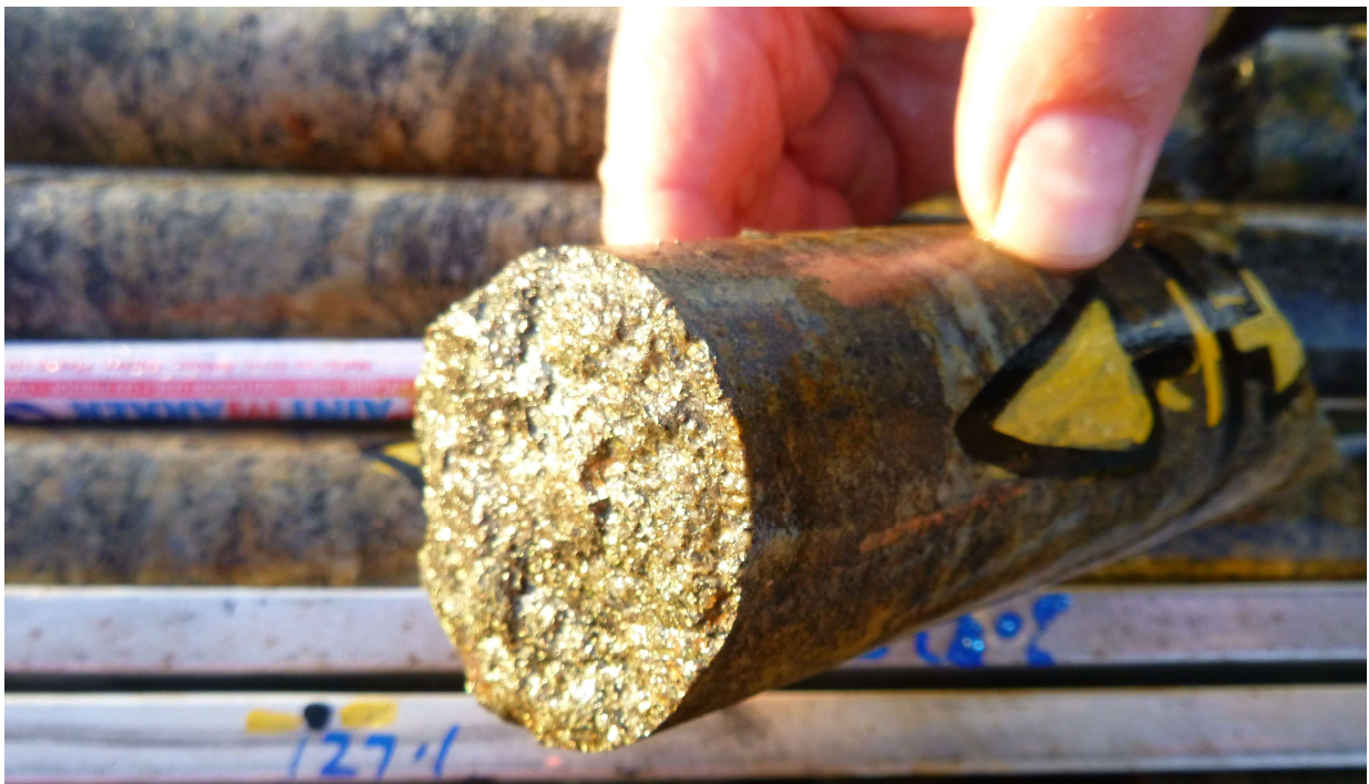
Figure 4: An example of the strongly pyritic bands in albitic gneiss in DD95STV3.
