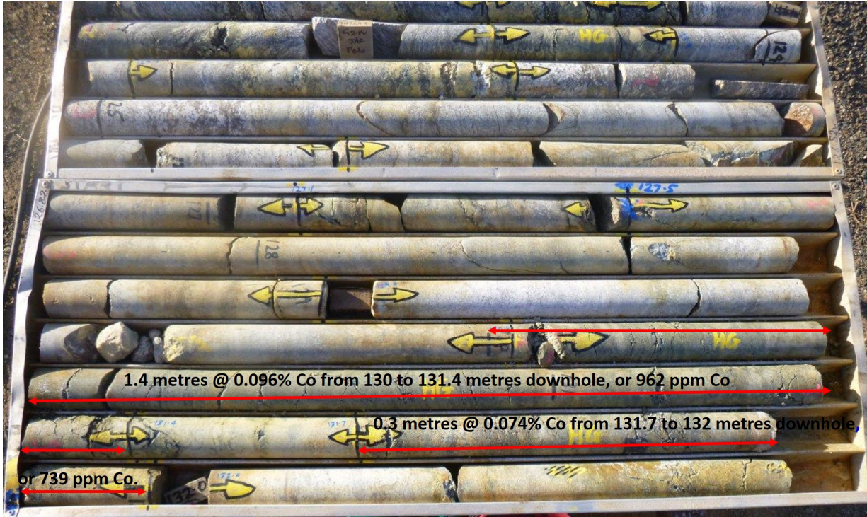
Figure 5: Pyrite zone in DD95STV3 from around 123 to 133 metres being relogged.
