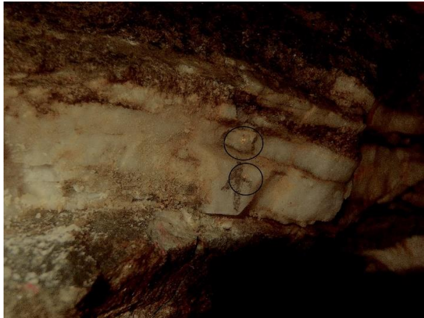
Photo 2. Gold in quartz in development face highlighted by annotated circles, correlating with gold seen in diamond drill core.
