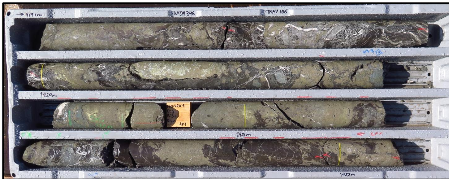
Figure 1 Shows Tray 106 from hole WFDH346 at 419.1m to 422.1m. Massive to semi-massive pyrite and chalcopyrite.
